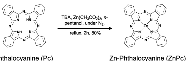
Fig. 4 Metalation reaction of Pc to produce ZnPc.
