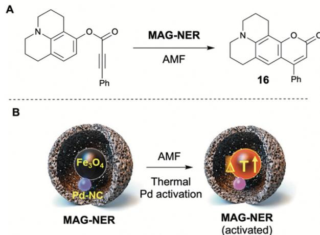
Fig. 12 (A) Formation of coumarin derivative **16** *via* **MAG-NER** catalyzed carbocyclization after catalyst activation using an alternating magnetic field (AMF). (B) Schematic representation of **MAG-NER** and its AMF activation mechanism.<sup>97</sup> Partly reproduced from ref. 97 with permission from ACS.
