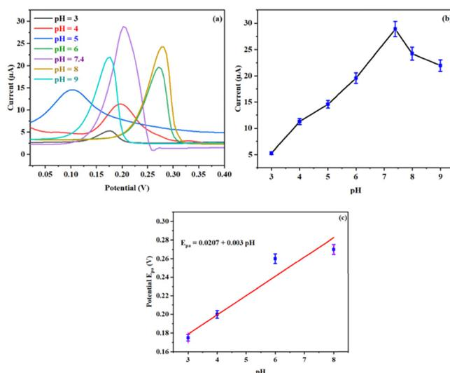
Fig. 8 (a) and (b) Effect of solution pH on the current response of creatinine at the  $[\text{Cu}_2\text{I}_2(\mu\text{-pyrazine})]/\text{GCE}$  electrode in 0.1 M phosphate buffer solution containing 100  $\mu\text{M}$  creatinine. (c) Inset: Linear plot of  $E_{\text{pa}}$  versus pH.
