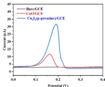
Fig. 7 Differential pulse voltammetry (DPV) of 100  $\mu\text{M}$  creatinine at the bare GCE, CuO/GCE and  $[\text{Cu}_2\text{I}_2(\mu\text{-pyrazine})]/\text{GCE}$  in 0.1 M phosphate buffer solution PBS (pH = 7.4).
