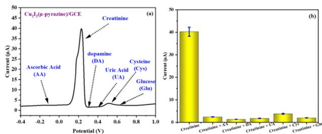
**Fig. 10** DPV responses of the  $[\text{Cu}_2\text{I}_2(\mu\text{-pyrazine})]/\text{GCE}$  electrode toward 100  $\mu\text{M}$  creatinine in 0.1 M phosphate buffer solution (PBS, pH 7.4), in the absence and presence of 100  $\mu\text{M}$  common interfering species (AA, UA, Cys, DA, and glucose).
