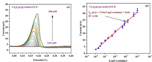
Fig. 9 (a) Differential pulse voltammetry (DPV) response of creatinine on various modified electrodes:  $[\text{Cu}_2\text{I}_2(\mu\text{-pyrazine})]/\text{GCE}$ , (b) corresponding calibration curves for creatinine using  $[\text{Cu}_2\text{I}_2(\mu\text{-pyrazine})]/\text{GCE}$  in 0.1 M phosphate buffer solution PBS pH = 7.4.
