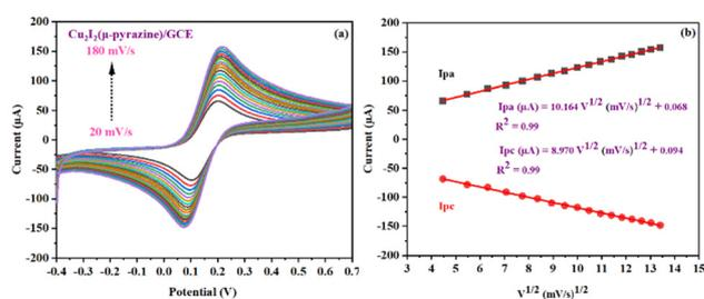
Fig. 6 (a) Cyclic voltammograms of the  $[\text{Cu}_2\text{I}_2(\mu\text{-pyrazine})]$ -modified electrode recorded in a 0.1 M KCl solution containing 5 mM  $[\text{Fe}(\text{CN})_6]^{3-/4-}$  at scan rates ranging from 20 to 180  $\text{mV s}^{-1}$ . (b) Inset: Plot of redox peak current as a function of the square root of the scan rate.
