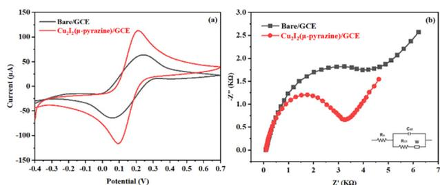
Fig. 5 (a) CV curves and (b) EIS spectra of bare/GCE and  $[\text{Cu}_2\text{I}_2(\mu\text{-pyrazine})]$ -modified GCE electrodes in a 5 mM  $[\text{Fe}(\text{CN})_6]^{3-/4-}$  solution containing 0.1 M KCl at a scan rate of 100  $\text{mV s}^{-1}$ , conducted over a frequency range of 0.05 Hz to 100 000 Hz with a 10 mV amplitude.
