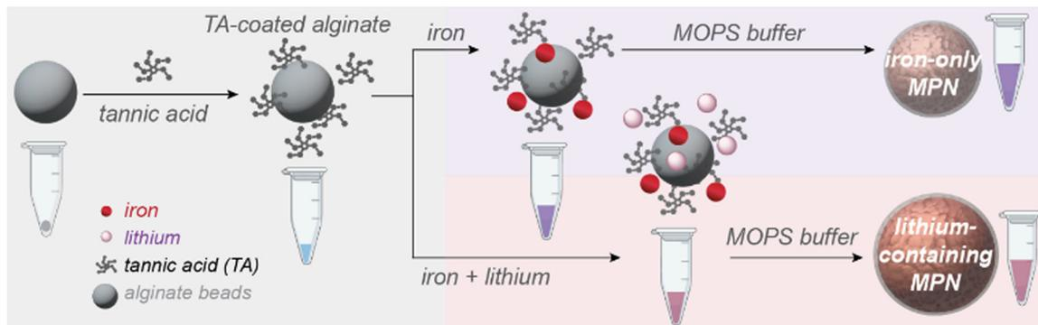
**Scheme 1** Preparation of MPN-coated alginate. Alginate beads are initially exposed to tannic acid (TA). To make iron-only MPNs, iron(III) chloride ( $\text{FeCl}_3$ ) is then added, followed by MOPS buffer to stabilize the network. To make lithium-containing MPNs, a pre-mixed solution of  $\text{FeCl}_3$  and  $\text{LiCl}$  is added to the TA-beads prior to MOPS addition.
