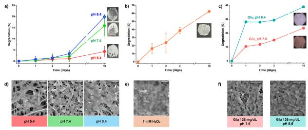
Fig. 6 %Degradation with digital images (a)–(c) and SEM images (d)–(f) of BE-PVA mats upon incubation at pH = 5.4, 7.4, and 8.4 (a) and (d), in 1 mM agueous  $H_2O_2$  solution (b) and (e), and in 126 mg dL<sup>-1</sup> agueous Glu solution with and without NaOH (c) and (f). Scale bars = 5 µm (d) and (f) and 2 µm (e).
