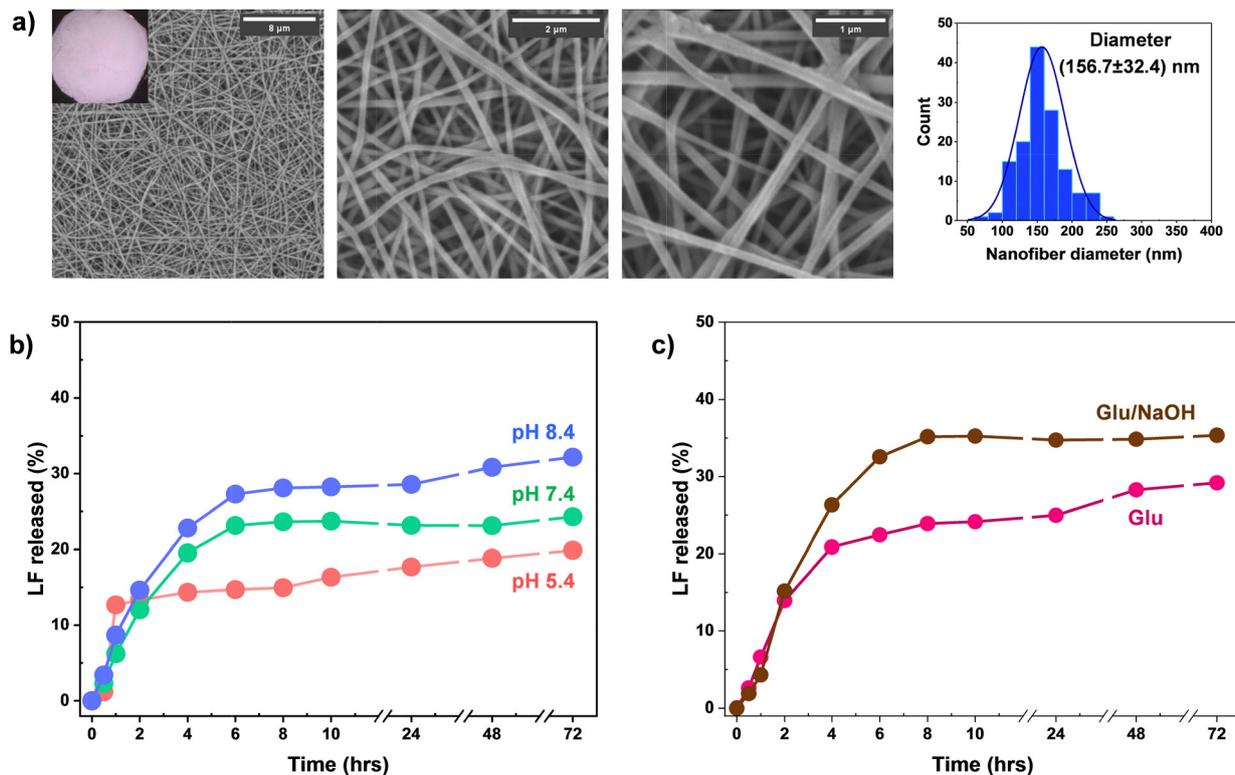
Fig. 7 SEM images with different magnifications and histogram of BE-PVA/LF mats (10 wt% loading) (a) and release profile of LF at different pH values (b) and in 126 mg dL<sup>-1</sup> Glu solution with and without NaOH (c).
