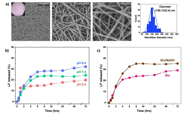
Fig. 7 SEM images with different magnifications and histogram of BE-PVA/LF mats (10 wt% loading) (a) and release profile of LF at different pH values (b) and in 126 mg  $dL^{-1}$  Glu solution with and without NaOH (c).
