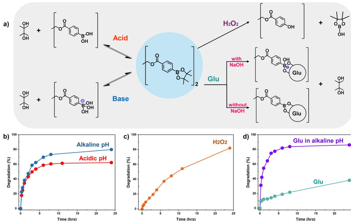
Fig. 5 Schematic illustration of DBA-EP degradation in response to HCl (acid), NaOH (base), H<sub>2</sub>O<sub>2</sub>, and Glu (a) and the %degradation over incubation time with HCl and NaOH (b), H<sub>2</sub>O<sub>2</sub> at BE/H<sub>2</sub>O<sub>2</sub> = 1/1 (c), and Glu with and without NaOH at BE/Glu = 1/1 (d).
