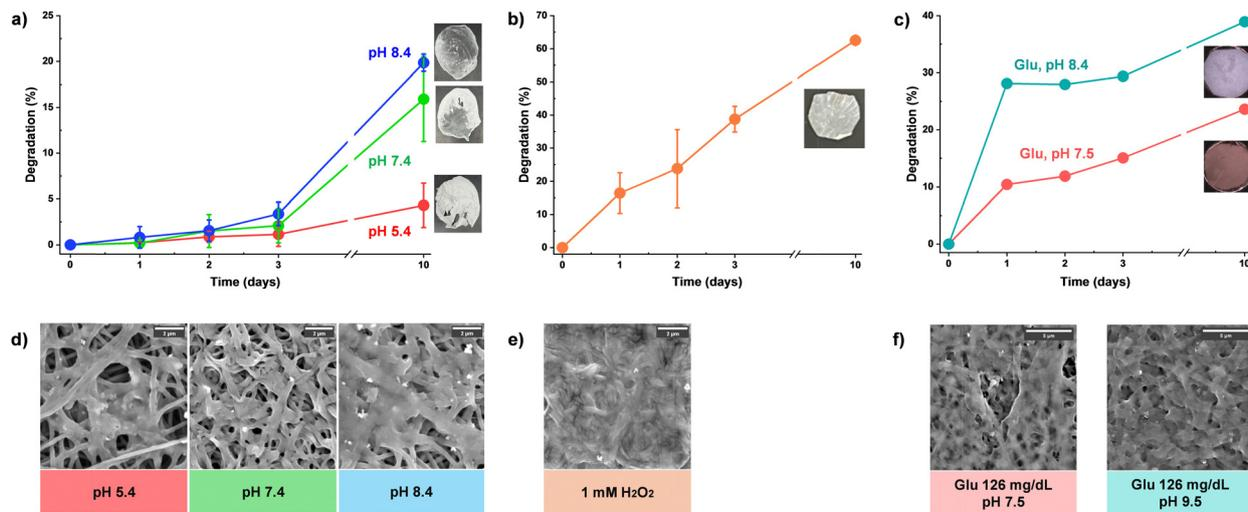
Fig. 6 %Degradation with digital images (a)–(c) and SEM images (d)–(f) of BE-PVA mats upon incubation at pH = 5.4, 7.4, and 8.4 (a) and (d), in 1 mM aqueous H<sub>2</sub>O<sub>2</sub> solution (b) and (e), and in 126 mg dL<sup>-1</sup> aqueous Glu solution with and without NaOH (c) and (f). Scale bars = 5  $\mu$ m (d) and (f) and 2  $\mu$ m (e).
