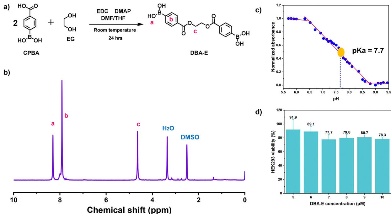
Fig. 2 For a new DBA-E phenyldiboronic acid crosslinker: synthesis exploring an EDC-mediated coupling reaction (a), <sup>1</sup>H NMR spectrum in DMSO-d<sub>6</sub> (b), spectroscopic titration curve of normalized absorbance at  $\lambda = 285$  nm over a pH range of 5.5–9.5 (c), and viability of HEK293 cells incubated for 24 h using a resazurin reduction assay (d).
