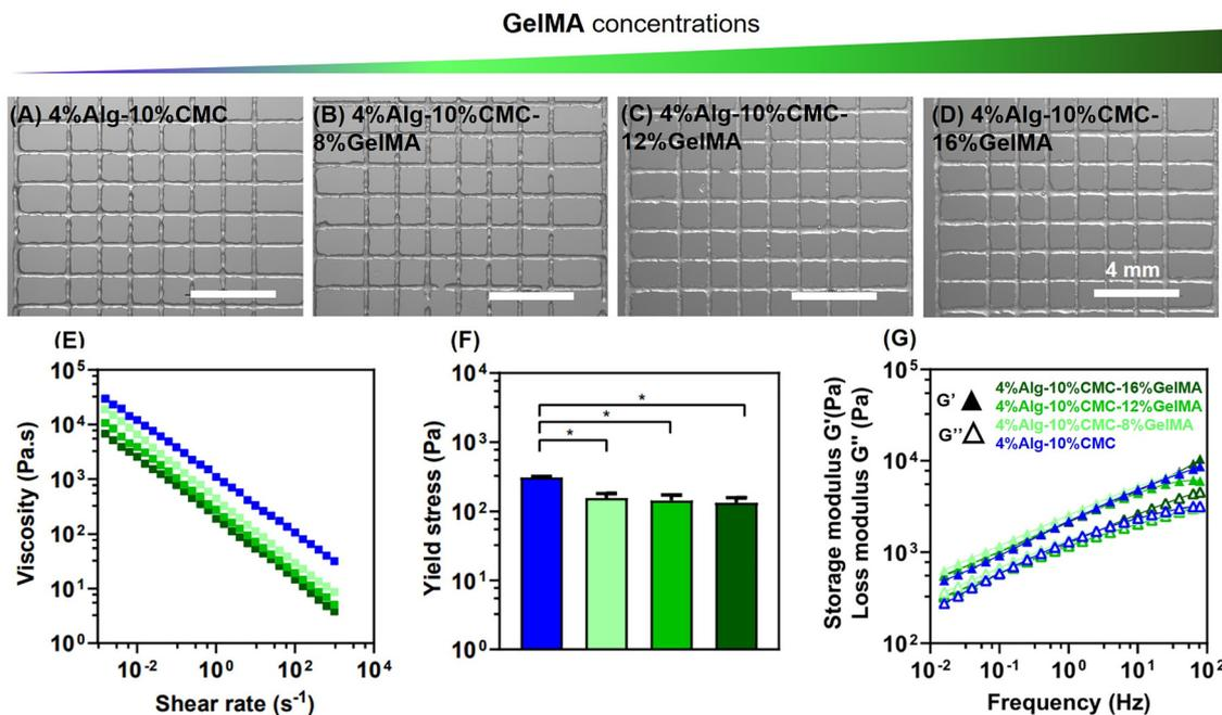
**Fig. 3** Correlation between printing and rheology of 4% Alg–10% CMC–GelMA. (A)–(D) Represent stereomicroscopic images of 3D-printed scaffolds. (E)–(G) Depict the inks' flow sweep, the yield stress deduced from amplitude sweep and frequency sweep, respectively.
