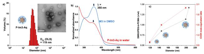
Fig. 4 For P-Im3-Aq nanogels in aqueous solution, DLS diagram with the TEM image (scale bar = 200 nm) as the inset (a); UV/vis spectrum at  $0.3 \text{ mg m}^{-1}$ . compared with that of M3 in DMSO (30 µM) (b); and evolution of diameter with varying amounts of DMSO and CI/OH mole equivalent ratio (c).
