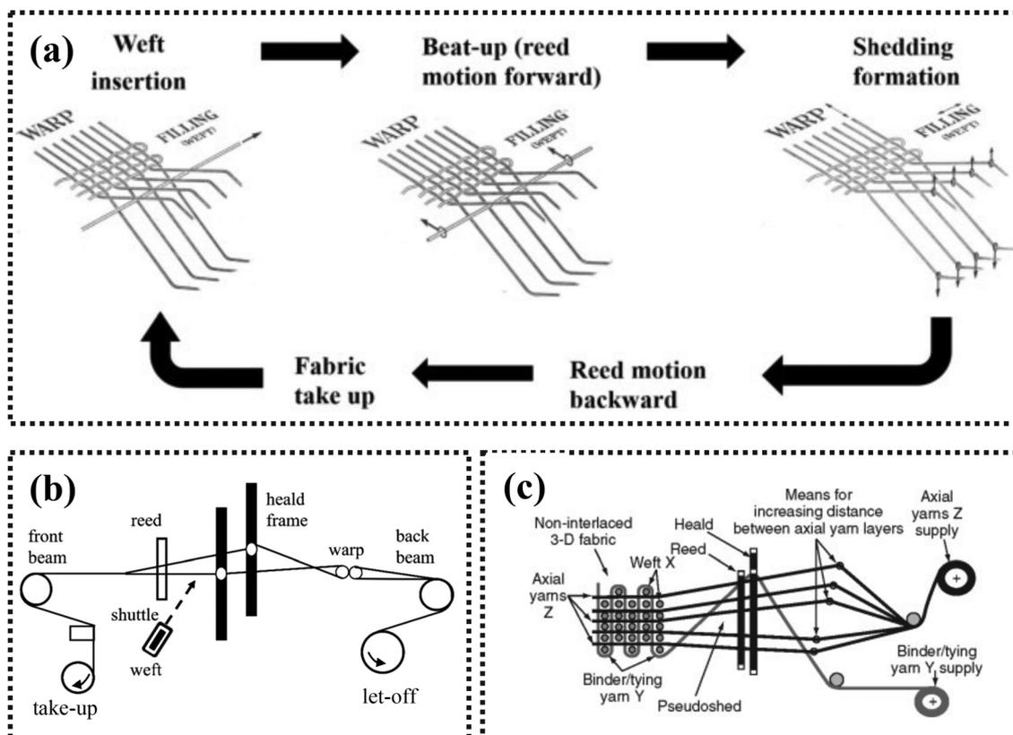
Fig. 2 Weaving processes. (a) A complete loom motion.<sup>105</sup> Reproduced with permission, copyright 2019, Elsevier. (b) 2D weaving process.<sup>106</sup> Reproduced with permission, copyright 2023, Sage Publications. (c) 3D weaving process.<sup>107</sup> Reproduced with permission, copyright 2008, Elsevier.
