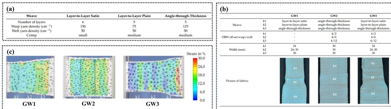
Fig. 8 Multilayer woven fabrics with different number of layers, warp density and crimps used for the artificial ligament.<sup>118</sup> Reproduced under the terms and conditions of the Creative Commons Attribution (CC BY) license. (a) Parameters of layer-to-layer satin, layer-to-layer plain and angle-through-thickness woven fabrics. (b) 3D gradient woven structures. (c) The strain in the individual zones of the gradient weave structures.
