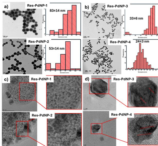
Fig. 2 Electron microscopy images with size distribution: (a) TEM images of Res-PdNP-1 and Res-PdNP-2, (b) TEM images of Res-PdNP-3 and Res-PdNP-4, (c) HRTEM images of Res-PdNP-1 and Res-PdNP-2 and (d) HRTEM images of Res-PdNP-3 and Res-PdNP-4.
