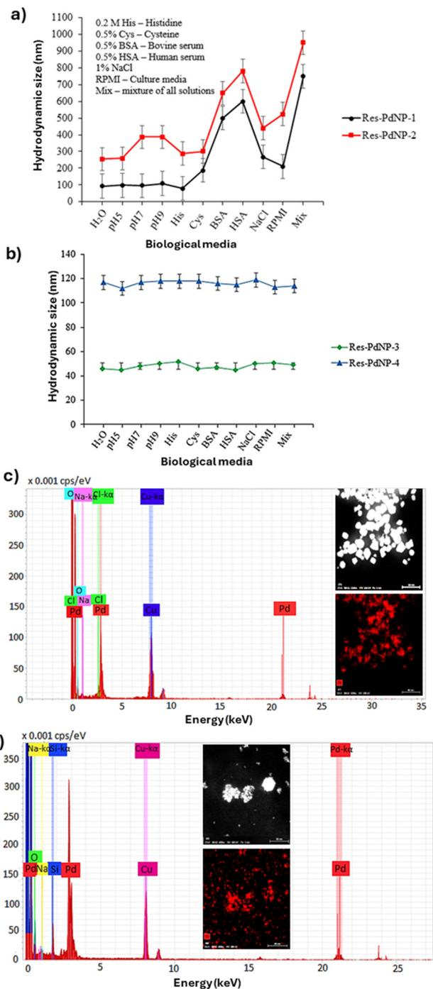
Fig. 4 *In vitro* stability and elemental analysis: (a) stability of Res-PdNP-1 and Res-PdNP-2, (b) stability of Res-PdNP-3 and Res-PdNP-4, (c) EDS of Res-PdNP-3 and (d) EDS of Res-PdNP-4 showing the presence of Pd. Res-PdNP-1 and Res-PdNP-2 not stable in BSA, HSA and mix media.
