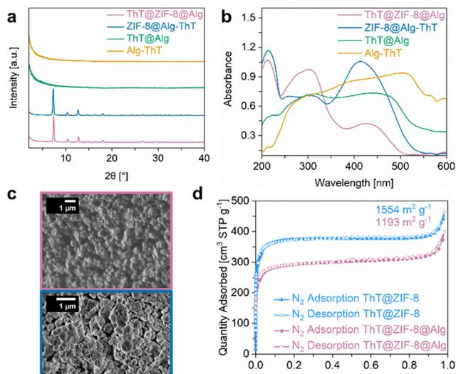
**Fig. 2** (a) Stacked PXRDs of ThT@ZIF-8@Alg (violet), ZIF-8@Alg-ThT (dark blue), ThT@Alg (green) and Alg-ThT (orange), (b) DR-UV/Vis spectra of ThT@ZIF-8@Alg, ZIF-8@Alg-ThT, ThT@Alg and Alg-ThT, (c) SEM images of ThT@ZIF-8@Alg (top) and ZIF-8@Alg-ThT (bottom), (d)  $N_2$  sorption isotherms (77 K) and calculated specific BET surface areas of ThT@ZIF-8 (light blue) and ThT@ZIF-8@Alg.
