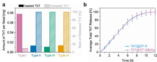
**Fig. 3** (a) Comparison of amounts of ThT integrated in (left columns, filled) or released from (right columns, dashed) ThT@ZIF-8@Alg, ZIF-8@Alg-ThT, ThT@Alg and Alg-ThT beads, (b) Averaged release profiles of ThT from triplicate series of ThT@ZIF-8 and ThT@ZIF-8@Alg in PBS (pH 6). The ThT@ZIF-8@Alg curve was normalised to the ThT amount in solution.
