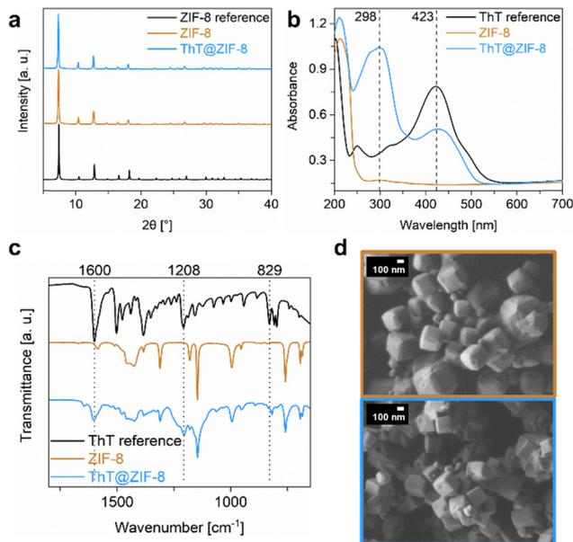
Fig. 1 (a) PXRDs of ZIF-8 (brown), ThT@ZIF-8 (blue) and a reference pattern of ZIF-8 (black, CCDC: 864309),<sup>52</sup> (b) DR-UV/Vis spectra of ZIF-8, ThT@ZIF-8 and ThT powder as reference (black), (c) FTIR spectra shown from 1800 to 650  $\text{cm}^{-1}$  of ZIF-8, ThT@ZIF-8 and ThT powder as reference, (d) SEM images of ZIF-8 (top) and ThT@ZIF-8 (bottom).
