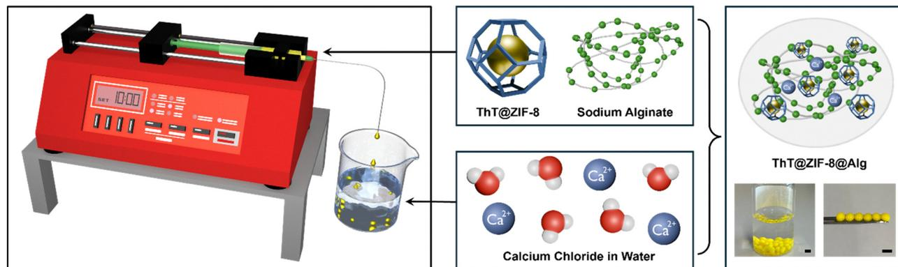
**Scheme 1** Schematic representation of the syringe pump setup for automated fabrication of ThT@ZIF-8@Alg beads with a uniform shape and size. A syringe filled with aqueous ThT@MOF/SA dispersion is fixed on a syringe pump and the content is steadily dropped into a  $\text{Ca}^{2+}$  curing solution, upon which the spherical beads are formed; scale bar = 2 mm.
