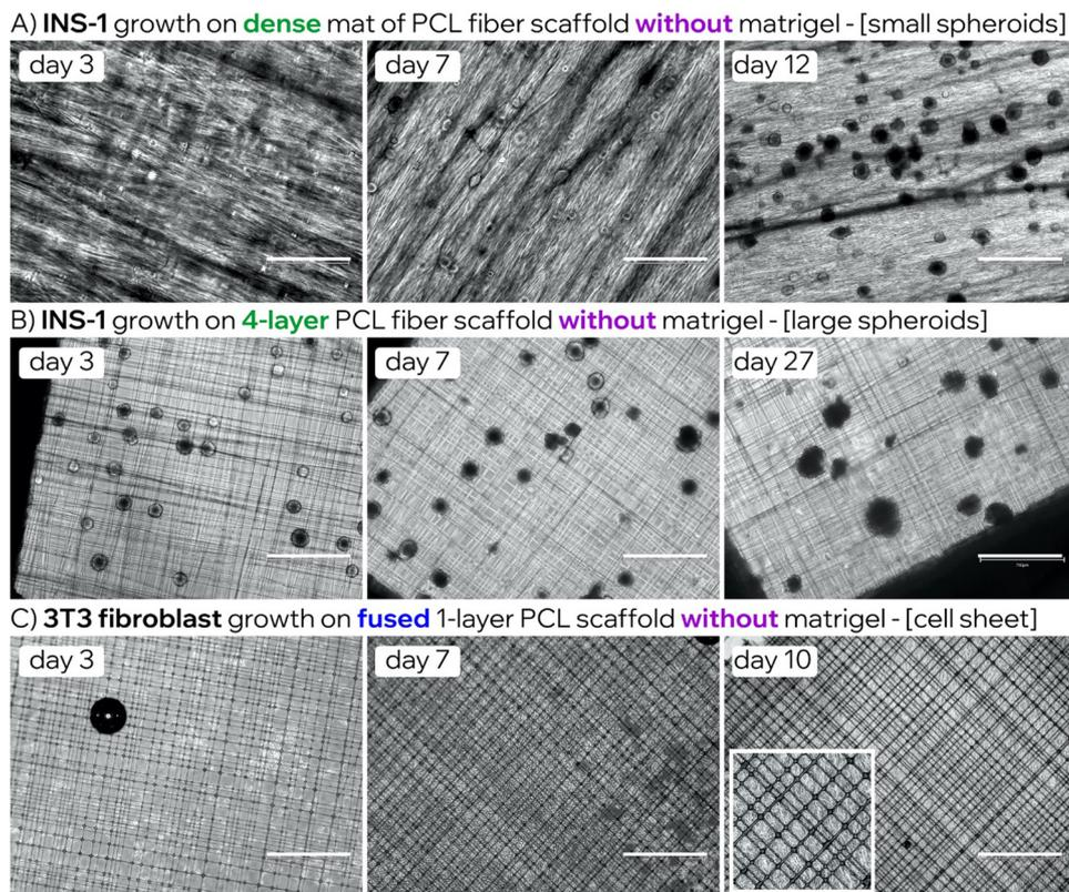
Fig. 6 Cell growth on different scaffolds. (A) INS-1 on the scaffold with densely packed fibers without Matrigel form numerous smaller spheroids. (B) INS-1 on the 4-layered scaffold with overlaid fibers without Matrigel form large spheroids. (C) 3T3 fibroblasts on 1-layered scaffold with fused fibers without Matrigel form a cell sheet structure on Day 7–10. Scale bars = 750  $\mu\text{m}$ .
