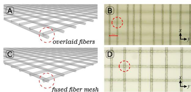
Fig. 3 Overlaid vs. fused PCL fiber mesh: (A) schematic of overlaid fibers in a crisscross layout; (B) optical microscope image of overlaid PCL fiber array with focus on y-axis-oriented fibers; (C) schematic of fused fiber mesh; (D) optical microscope image of overlaid PCL fiber array with focus on y-axis-oriented fibers.
