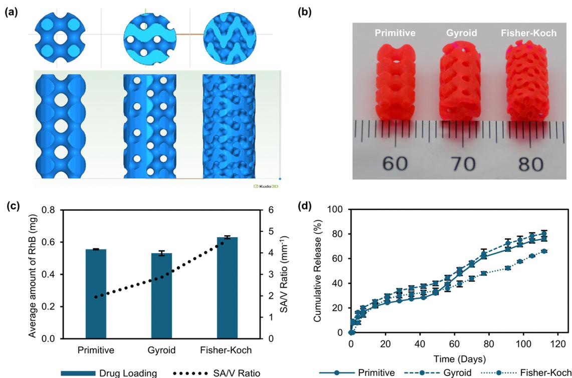
**Fig. 7** Characterization of lattice type series. (a) CAD models of lattice devices. (b) Visible light photographs of 3 mm unit cell primitive, gyroid, and Fisher–Koch lattices, from left to right. (c) Drug loading and SA/V ratio of different lattices. (d) Cumulative release of RhB from lattice type series ( $n = 3$ ). Error bars represent one standard deviation.
