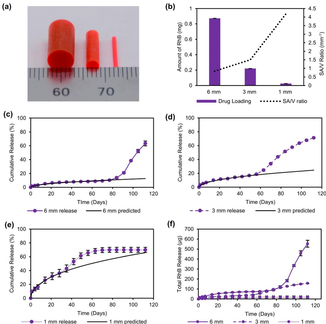
Fig. 3 *In vitro* release from diameter series. (a) Images of cylinders. (b) Drug loading and SAV ratios of cylinders with different diameters. Comparison of actual and predicted RhB release from (c) 6 mm, (d) 3 mm, and (e) 1 mm cylinders. The predicted drug release if assuming simple radial diffusion from the cylinders and that the drug release profiles follow a simple diffusion model. (f) Total amount of RhB released from cylinders ( $n = 3$ ). Error bars represent one standard deviation.
