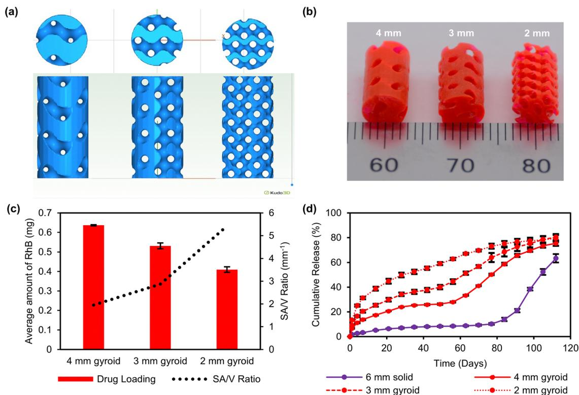
Fig. 5 Characterization of unit cell series. (a) CAD models of lattice devices. (b) Visible light photographs of 4 mm, 3 mm, and 2 mm unit cell gyroid lattices, from left to right. (c) Drug loading and SAV ratio of different lattices. (d) Cumulative release of RhB from unit cells series compared to 6 mm solid cylinder ( $n = 3$ ). Error bars represent one standard deviation.
