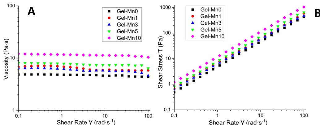
Fig. 2 Viscosity vs. shear rate (A) and shear stress vs. shear rate (B) of all polyphosphate coacervate gels.
