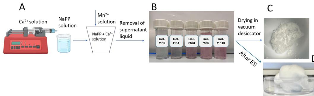
Fig. 1 (A) Schematic of the synthesis of PGs *via* coacervation; (B) images of all coacervate gels; (C) PGP-Mn0 in the system  $P_2O_5$ -CaO- $Na_2O$  obtained after drying of the coacervate Gel-Mn0 in a vacuum desiccator; (D) cotton-like bundle of PGF-Mn0 after ES of Gel-Mn0.
