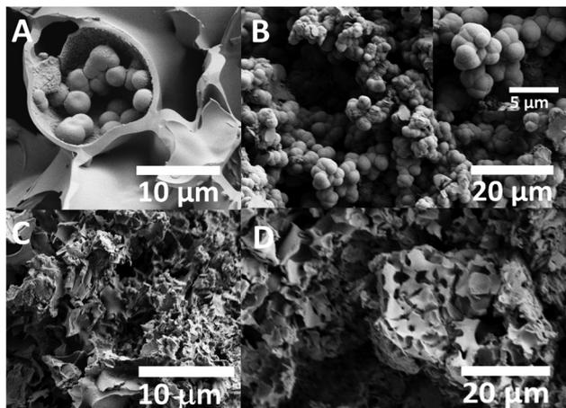
Fig. 11 SEM micrographs of PGP-Mn1 after immersion in CM for 24 h (A) and 72 h (B) and after immersion in Tris-B for 24 h (C) and 72 h (D).
