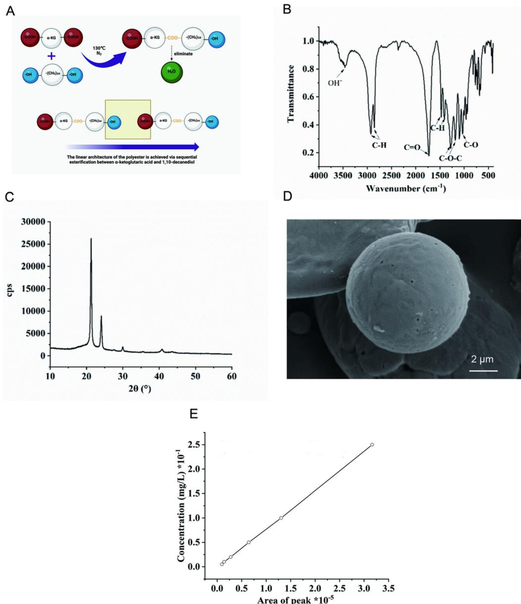
Fig. 1 Characterization of  $\alpha$ -KG polyester microspheres. (A) Polyester formation process. (B) Fourier transform infrared spectroscopy for  $\alpha$ -KG Polyester Microspheres. (C) XRD analysis. (D) SEM. (E) The  $\alpha$ -KG release standard curve. (E) Schematic diagram of the synthesis of  $\alpha$ -KG Polyester.
