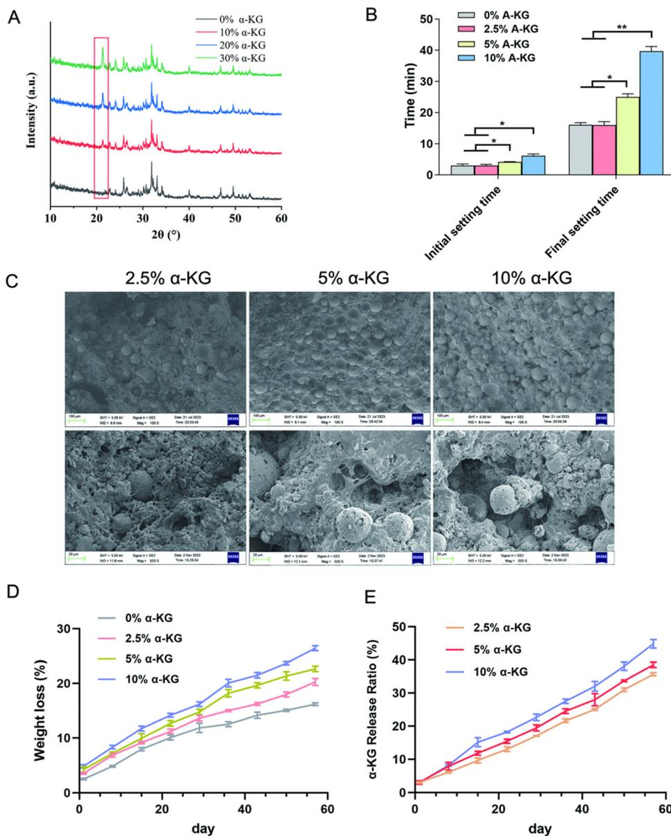
Fig. 2 Characterization of the CPC/ $\alpha$ -KG. (A) XRD analysis. (B) Initial and final setting times of the CPC/ $\alpha$ -KG. (C) SEM of the CPC/ $\alpha$ -KG. (D) Degradation curve of the CPC/ $\alpha$ -KG *in vitro*. (E)  $\alpha$ -KG release curves of bone cement composed of 2.5%, 5%, and 10 wt%  $\alpha$ -KG microspheres. Data are presented as mean  $\pm$  SD ( $n = 3$ ); \* $p < 0.05$ , \*\* $p < 0.01$ , \*\*\* $p < 0.001$ .
