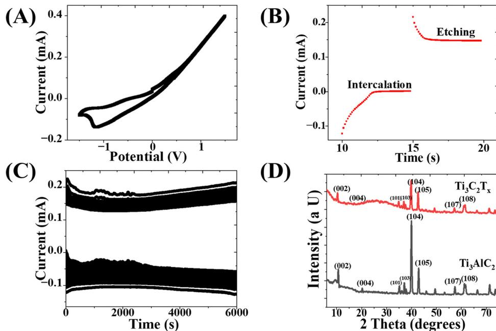
Fig. 2 (A) Cyclic voltammety curve for the  $Ti_3AlC_2$  MAX electrode at a potential window of  $-1.5$  V to  $+1.5$  V, (B) a representation of the chronoamperometry curve for 5 s each at potentials of  $-0.6$  V (intercalation) and  $+0.6$  V (etching), (C) chronoamperometry including both intercalation and etching for 6000 s and (D) XRD analysis for the pristine  $Ti_3AlC_2$  Max phase and  $Ti_3C_2T_x$  MXene.
