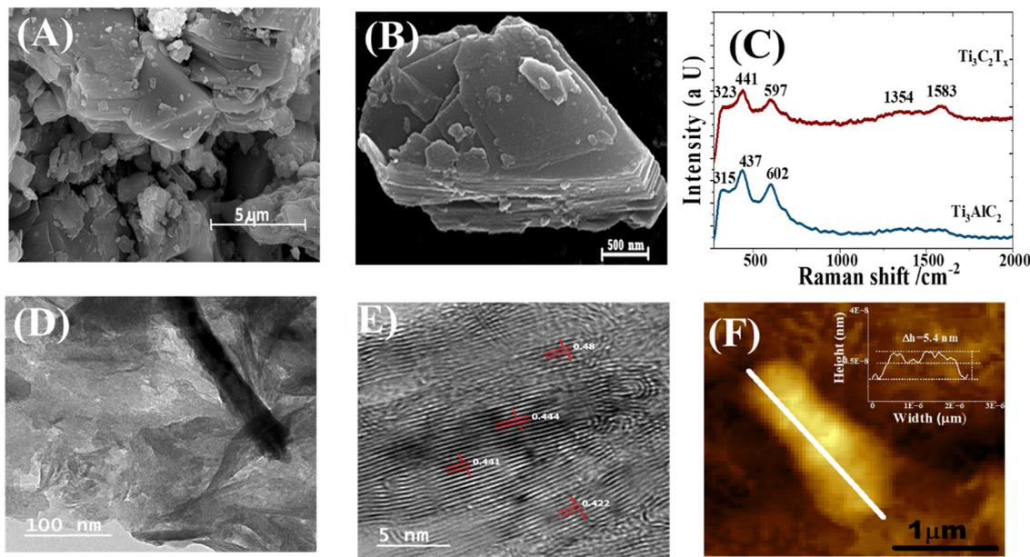
Fig. 3 SEM images for (A) the pristine  $\text{Ti}_3\text{AlC}_2$  MAX phase and (B)  $\text{Ti}_3\text{C}_2(\text{O,Cl})$  MXene; (C) Raman analysis for  $\text{Ti}_3\text{AlC}_2$  and  $\text{Ti}_3\text{C}_2(\text{O,Cl})$ ; (D) TEM images for  $\text{Ti}_3\text{C}_2(\text{O,Cl})$  MXene at 100 nm; (E) TEM image of  $\text{Ti}_3\text{C}_2(\text{O,Cl})$  at 5 nm and (F) AFM image of  $\text{Ti}_3\text{C}_2(\text{O,Cl})$  with a height of 5.4 nm.
