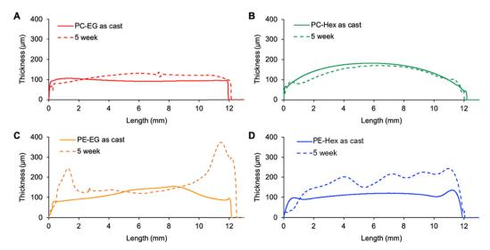
Fig. 6 Thickness of the poly(pro-E2) films: (A) PC-EG, (B) PC-Hex, (C) PE-EG, and (D) PE-Hex before and after incubation in PBS at 37 °C for 5 weeks.
