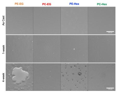
Fig. 7 SEM images of the four polymer films as-cast and after 1- and 4-weeks incubation (37 °C, PBS). In all images, the scale bar is 250 µm.
