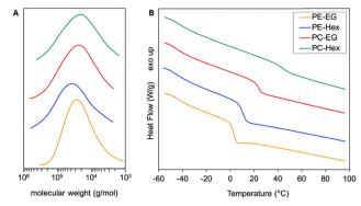
Fig. 2 Characterization of poly(pro-E2) materials. (A) Molecular weight distribution by gel permeation chromatography (GPC) and (B) thermal transitions quantified by differential scanning calorimetry (DSC).
