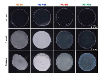
Fig. 5  $\,$  Photos of poly(pro-E2) films incubated at 37  $^{\circ}\text{C}$  in PBS (in the wet state) for 1 and 5 weeks.
