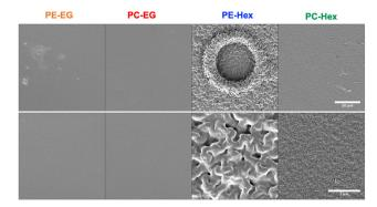
Fig. 8 Scanning electron microscopy images for surface characterization of submerged poly(pro-E2) films after 5-week incubation (37 °C, PBS) at two different magnifications. The scale bars are 20  $\mu$ m for the upper row and 5 µm for the lower row
