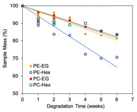
Fig. 4 Mass loss characterization of drop-cast poly(pro-E2) films at 60  $^{\circ}\text{C}$  in PBS.
