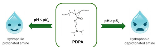
Fig. 2 Schematic illustration of the solubility of PDPA in aqueous medium according to solution pH.
