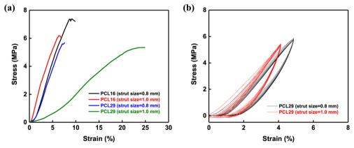
Fig. 6 Representative uniaxial compression test curves for 3D printed hybrid scaffolds of PCL16 and PCL29 (organic/inorganic: 70/30), printed with strut sizes of 0.8 mm and 1.0 mm (left), and cyclic compression test curves of the 3D printed hybrid PCL16 scaffolds (right).
