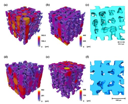
Fig. 5 µCT imaging and analysis of PCL29 3D printed scaffolds. Colour map to visualize the channel size of PCL29 scaffolds prepared with strut size 0.8 mm (a) and 1.0 mm (d); colour map to visualize the interconnecting channel thickness of PCL29 scaffolds prepared with strut size 0.8 mm (b) and 1.0 mm (e); sub-volumes of interest ( $2000 \times 2000 \times 2000 \mu m$ ) of PCL29 scaffolds prepared with strut size 0.8 mm (c) and 1.0 mm (f).
