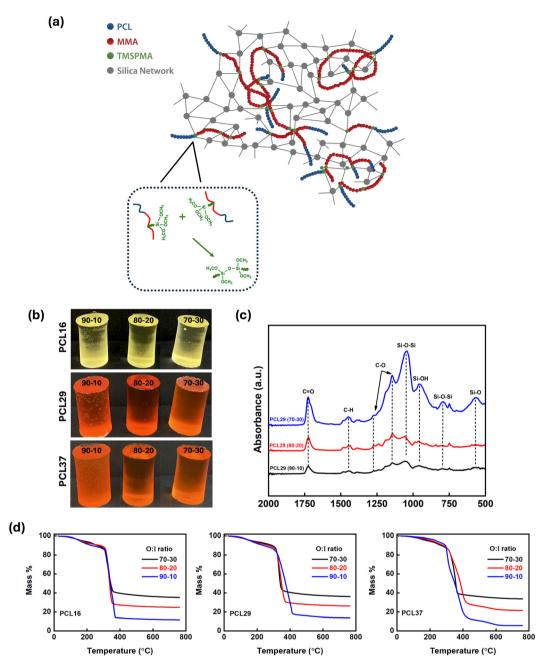
Fig. 2 (a) Schematic illustration of the formation of PCL-b-P(MMA-co-TMSPMA)/silica hybrids; (b) photographs of hybrid monoliths prepared using each the PCL-b-P(MMA-co-TMSPMA) copolymers (Table 1) and organic/inorganic (O:I) ratios 90:10, 80:20 and 70:30; (c) FTIR spectra of the hybrids prepared with PCL29 copolymer; (d) TGA thermograms of hybrids monoliths for all 3 PCL-b-P(MMA-co-TMSPMA) copolymers.
