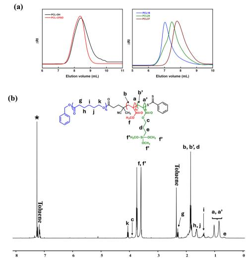
Fig. 1 (a) SEC chromatograms of PCL-OH and PCL-CPAD precursors (left) and of all PCL-b-P(MMA-co-TMSPMA) copolymers synthesized (right) Sample codes are explained in Table 1; (b) <sup>1</sup>H-NMR spectrum of PCL-b-P(MMA-co-TMSMPA)-2, PCL29, in CDCl<sub>3</sub>
