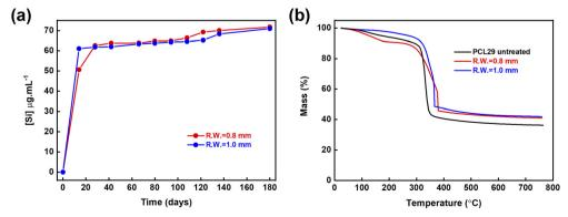
Fig. 7 (a) Si release of PCL29 (organic/inorganic: 70/30) 3D printed scaffolds (Strut size 0.8 mm and 1.0 mm) in PBS as a function of time, over the course of 180 days (ICP), (b) TGA graphs of PCL29 (organic/inorganic: 70/30) 3D printed scaffolds (Strut size 0.8 mm and 1.0 mm) after the exposure to PBS.
