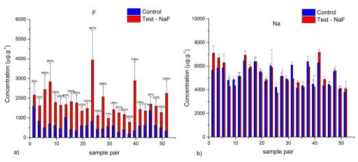
Fig. 1 Comparison of the (a) fluorine and (b) sodium concentration obtained for all the studied samples. Error bars correspond to the maximum deviation to the average value for the three measurements.
