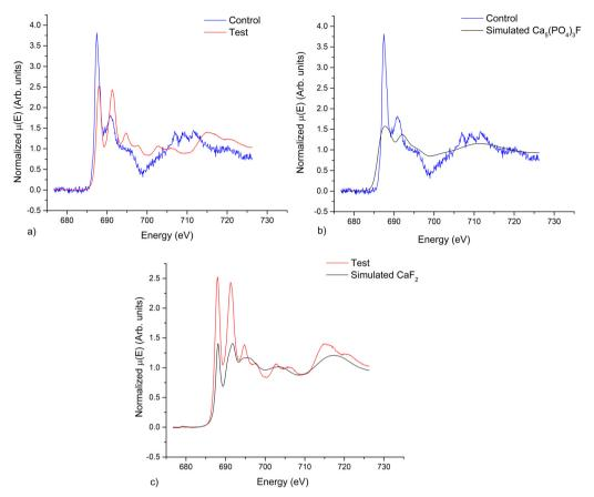
Fig. 2 Comparison of the NEXAFS spectra at the F K-edge obtained for (a) the control and test groups, and (b) the control group and simulated spectrum of Ca<sub>5</sub>(PO<sub>4</sub>)<sub>3</sub>F and (c) the test group and simulated spectrum for CaF<sub>2</sub>.
