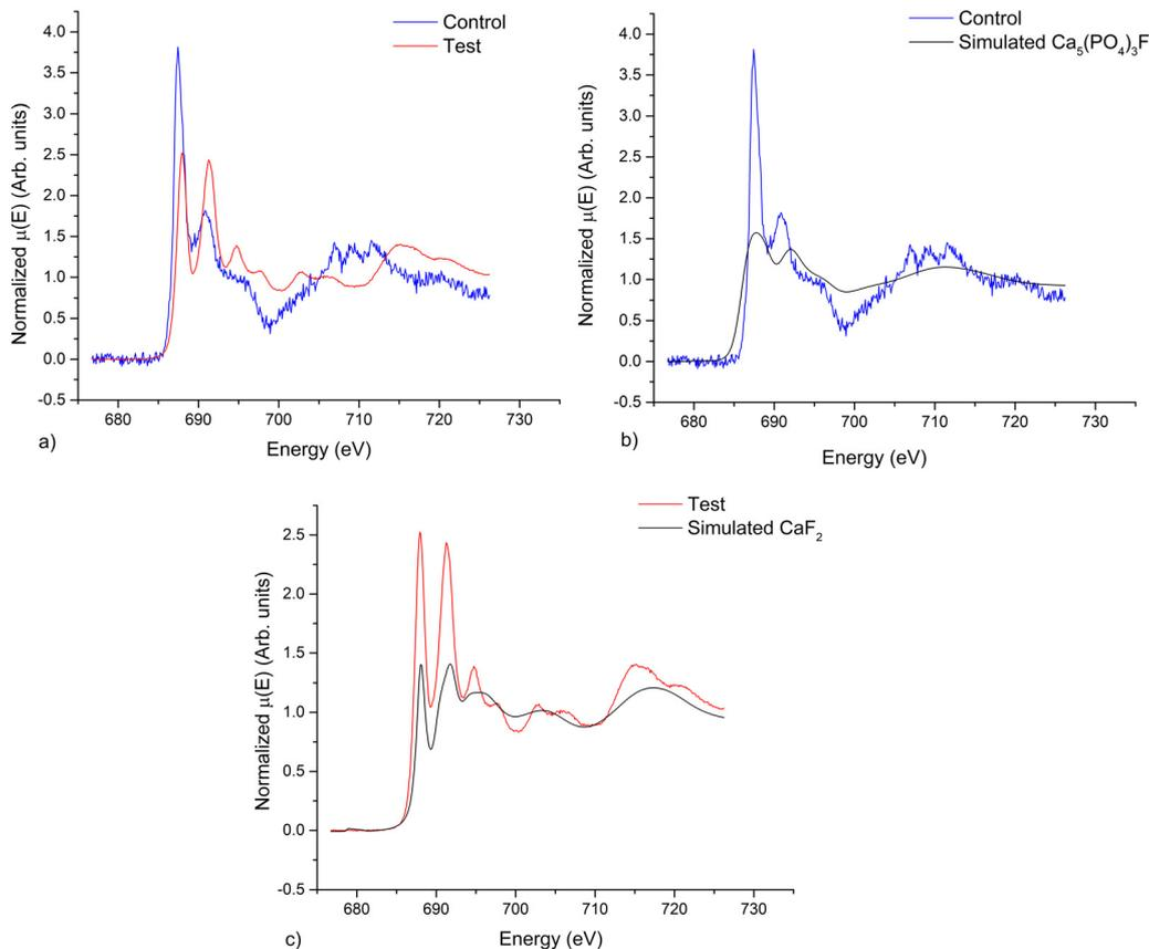
Fig. 2 Comparison of the NEXAFS spectra at the F K-edge obtained for (a) the control and test groups, and (b) the control group and simulated spectrum of  $\text{Ca}_5(\text{PO}_4)_3\text{F}$  and (c) the test group and simulated spectrum for  $\text{CaF}_2$ .
