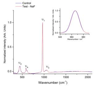
Fig. 4 Comparison of the Raman spectra for the control and test samples. As an inset, it is highlighted the slight shift for the symmetric stretching band of phosphate.
