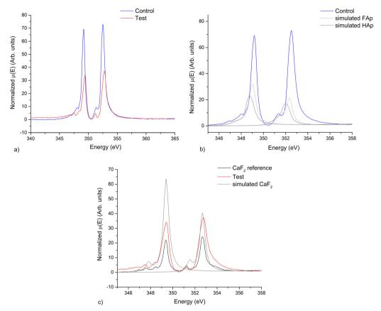
Fig. 3 Comparison of the NEXAFS spectra at the Ca L-edge obtained for (a) the control and test groups, (b) the control group, Hap and Fap simulated spectra and (c) the test group, CaF2 reference sample and simulated spectrum.
