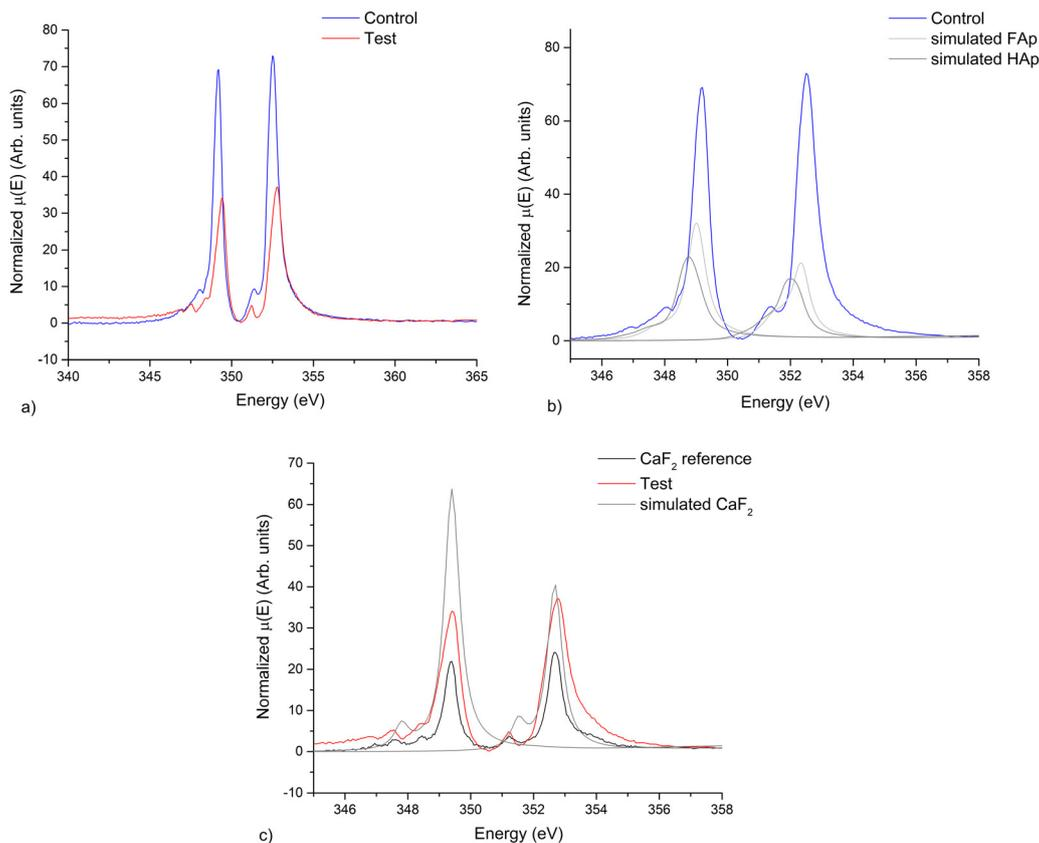
Fig. 3 Comparison of the NEXAFS spectra at the Ca L-edge obtained for (a) the control and test groups, (b) the control group, Hap and Fap simulated spectra and (c) the test group, CaF<sub>2</sub> reference sample and simulated spectrum.
