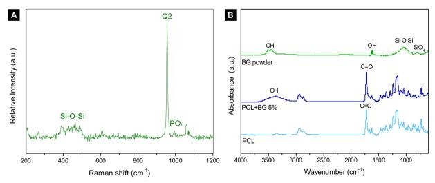
Fig. 2 (A) Raman spectrum of BG powder; (B) FTIR graph of BG powder, PCL, and PCL + BG5% indicating the chemical stretches present in each group.
