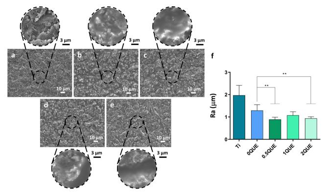
Fig. 1 SEM micrographs of (a) Ti, (b) 0QUE, (c) 0.5QUE, (d) 1QUE and (e) 2QUE with their respectively ampliations. Roughness is shown as the arithmetic average roughness parameter ( $R_a$ ) (f). The asterisks ( $p \le 0.01$  (\*\*)) indicate statistically significant differences for the QUE-doped coatings in comparison with OQUE. Results are shown as mean  $\pm$  SD.
