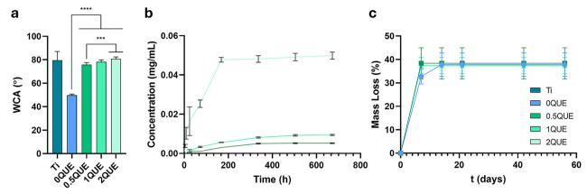
Fig. 3 Contact angle measurements (WCA; (a)), release kinetics of QUE (mg mL $^{-1}$ ) (b) and hydrolitic degradation results (c). The asterisks ( $p \le 0.001$  (\*\*\*) and  $p \le 0.0001$  (\*\*\*\*)) indicate statistically significant differences between the QUE-doped coatings and the OQUE. Results are shown as mean  $\pm$  SD.
