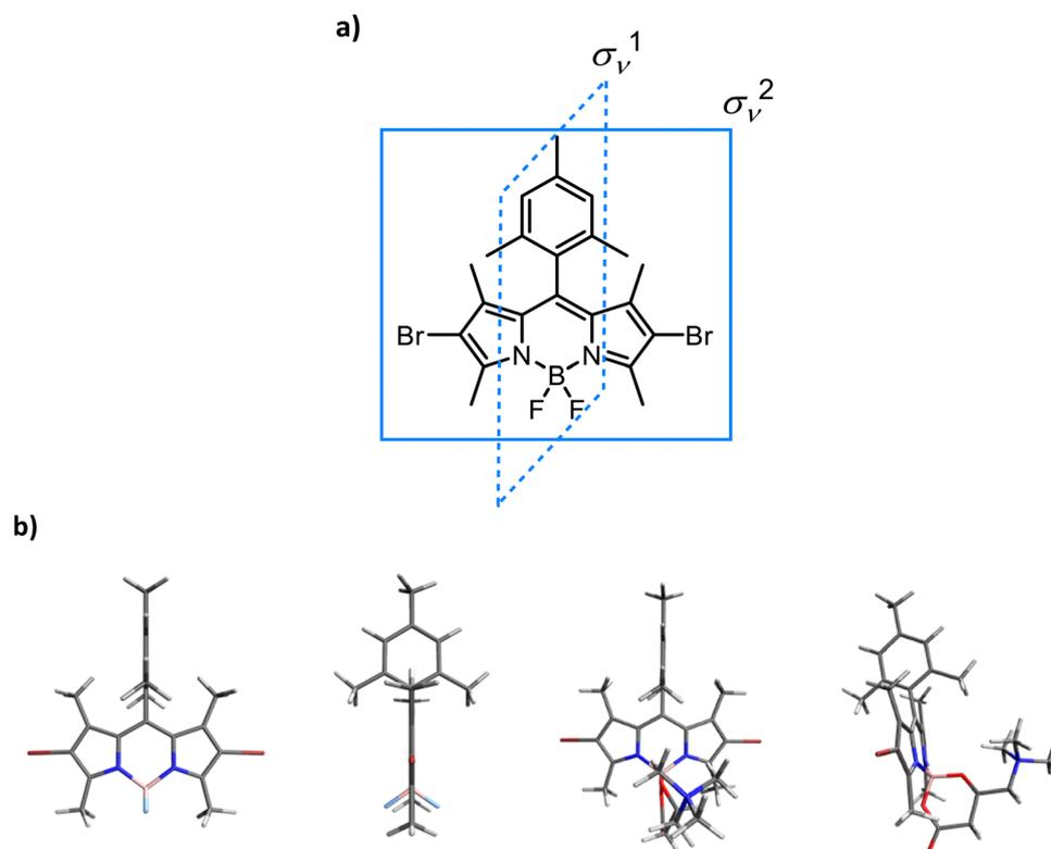
**Fig. 3** (a) Compound **3** with symmetry planes  $\sigma_v^1$  and  $\sigma_v^2$ . (b) Ground state structures optimized at the CAM-B3LYP/cc-pVDZ level of compounds **3** (left) and **1** (right), with perspective views along planes  $\sigma_v^1$  and  $\sigma_v^2$ , showing the symmetric and planar structure of probe **3** versus the non-planar structure of probe **1**.
