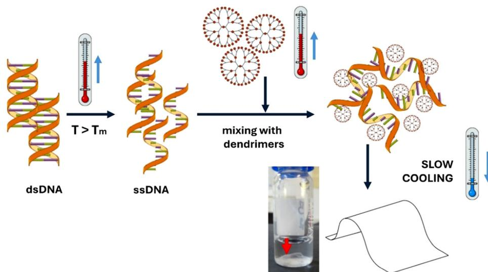
Fig. 1 General strategy followed for the preparation of hybrid DNA/dendrimer-based films. The dsDNA and dendrimers are first heated separately above the dsDNA melting temperature ( $T_m$ ), then mixed, and subsequently subjected to a slow cooling process.
