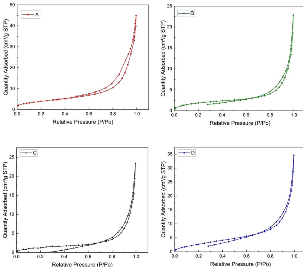
Fig. 5 Nitrogen adsorption-desorption isotherms for (A) free CuO nanoparticles, (B) *cis*@CuO, (C) *neda*@CuO, and (D) *oxa*@CuO.
