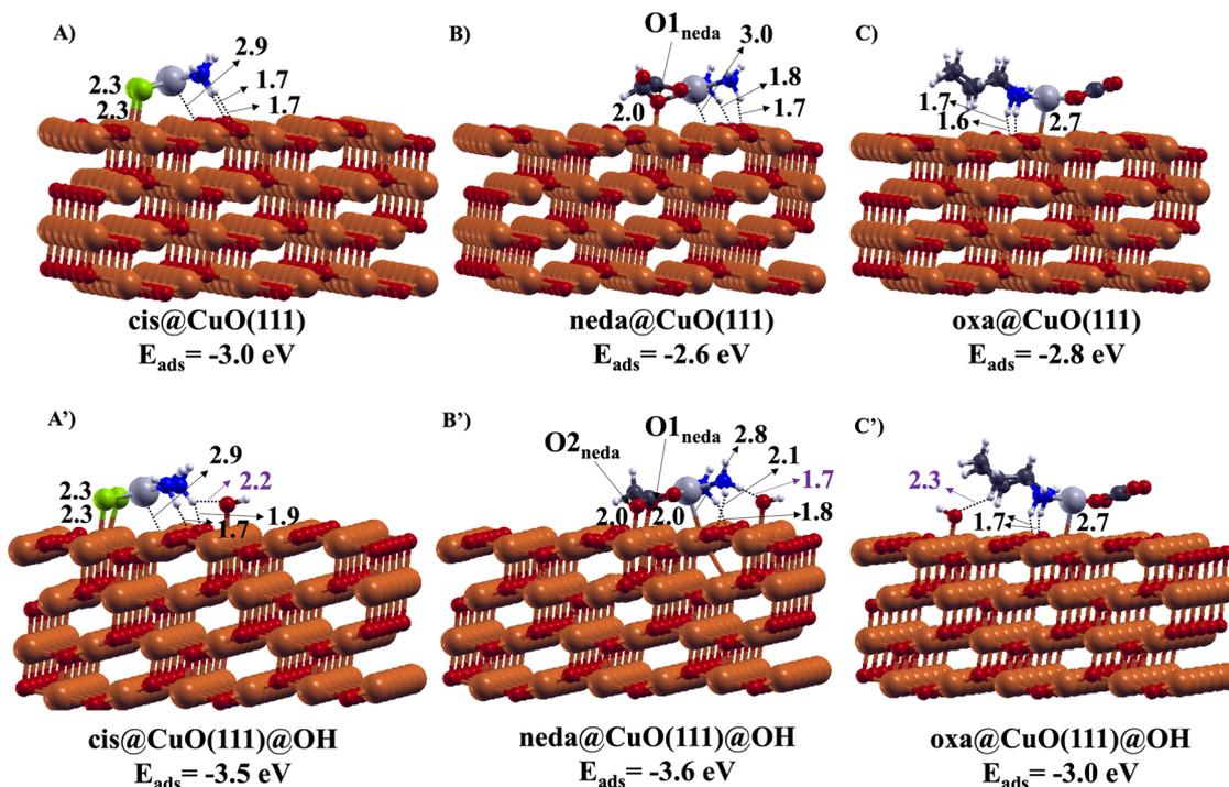
Fig. 12 Optimized geometries related to the interaction of cisplatin, nedaplatin and oxalipatin with CuO(111) (panels A–C) and CuO(111)@OH (panels A'–C') and the corresponding  $E_{\text{ads}}$  (eV). Cu, O, Cl, Pt, C, H and N atoms are represented in ball and sticks and depicted in auburn, red, green, gray, black, white and blue, respectively.
