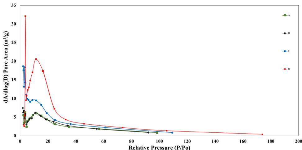
Fig. 8 BJH desorption  $dA/d\log(D)$  pore area vs relative pressure curves. (A)–(C) correspond to the samples *cis*@CuO, *neda*@CuO and *oxa*@CuO, respectively, whereas (D) is to the free CuO nanoparticles.
