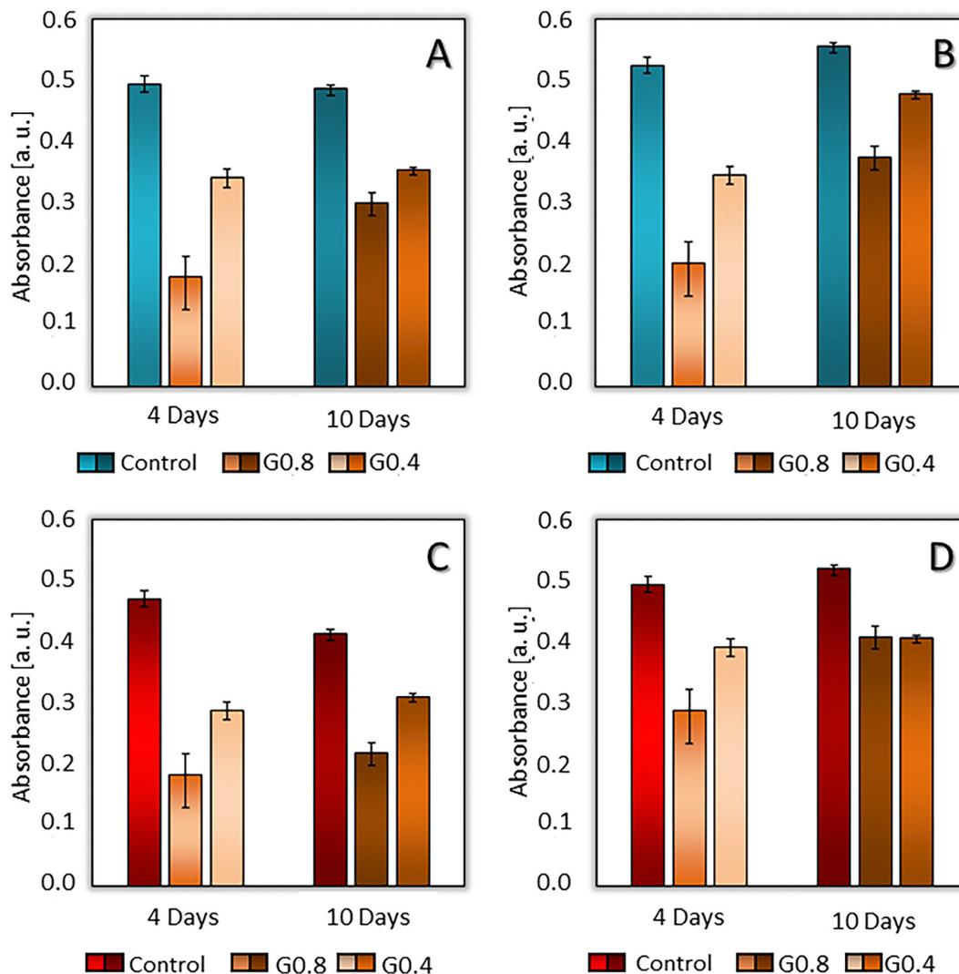
Fig. 6 Comparison of the antioxidant properties of modified PAC materials depending on the length of crosslinking time. (A) cPHC<sub>1</sub>:1, (B) cPHC<sub>2</sub>:3, (C) cPOC<sub>1</sub>:1, (D) cPOC<sub>2</sub>:3. Absorbance was measured at 517 nm.
