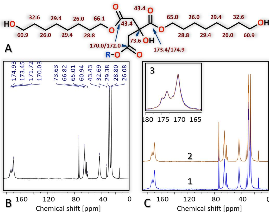
Fig. 3 Fragment of POC prepolymer structure along with chemical shift assignments based on <sup>13</sup>C MAS NMR analysis (A), <sup>13</sup>C MAS NMR spectra obtained for the cPOC\_2:3\_4d\_C with chemical shift assignments of the observed signals (B) and comparison of cPOC\_2:3\_4d\_C and cPOC\_2:3\_4d\_G0.8 spectra (C1) and (C2) and a close-up of the superimposed integrals of the carboxylic acid region of both spectra (C3).
