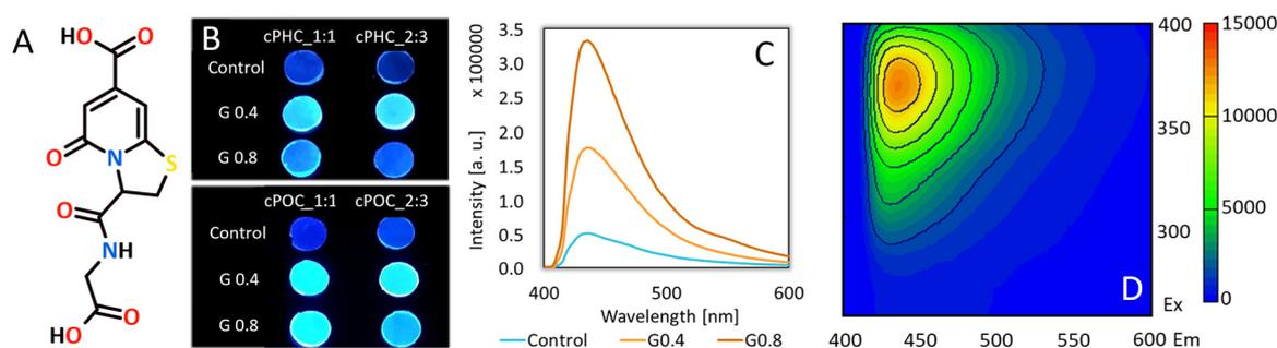
Fig. 4 The structure of CTPC fluorophore (A),<sup>47</sup> samples of control and modified cPAC materials under a UV lamp (B), photoluminescence (PL) emission spectra for control and modified cPHC\_1:1\_10d materials (C), and 3D fluorescence map for cPHC\_1:1\_10d\_G0.8 (D).
