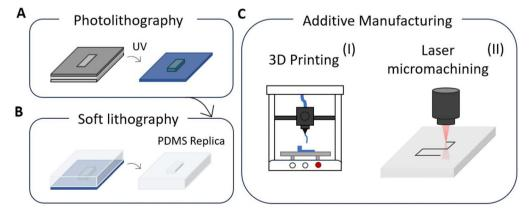
Fig. 7 Graphical schemes for the most used techniques in the context of microfluidic device production. Main representative lithographic based methods such as photolithography (A) for resolved master mold prototyping and soft lithography (B) for producing PDMS-based microchips. (C) Additive manufacturing approaches divided in 3D printing (I) based on layer-by-layer material deposition and laser micromachining (II) by femtosecond laser irradiation and chemical etching
