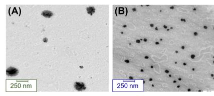
Fig. 3 Energy-filtered transmission electron microscopy images of PCL-PRoX1 (A) and PCL-PRoX2 (B).
