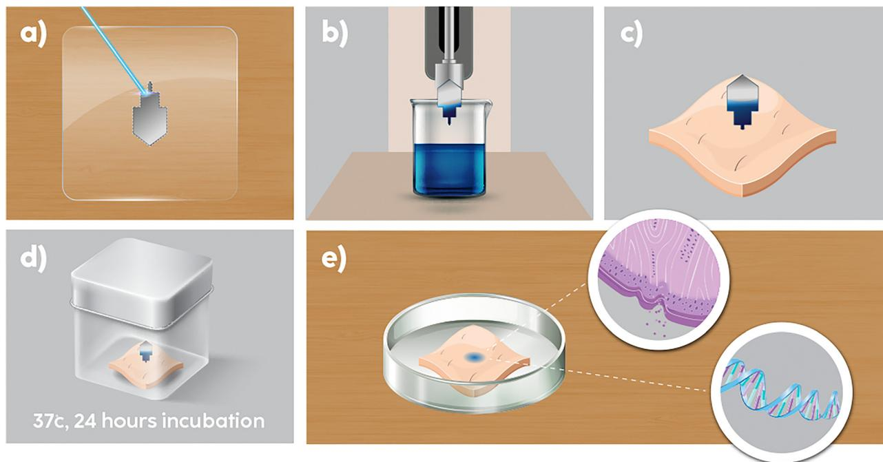
**Fig. 1** Experimental procedures. (a) PMMA sheet laser cut into microneedle. (b) Microneedle tip dipped into PEDOTs solutions. (c) PEDOT coated microneedle tip is implanted into excised, fresh human skin. (d) Sample incubated in water bath at 37 deg for 24 hours. (e) Skin in contact with PEDOT coated MN was processed for histology and RT-PCR.
