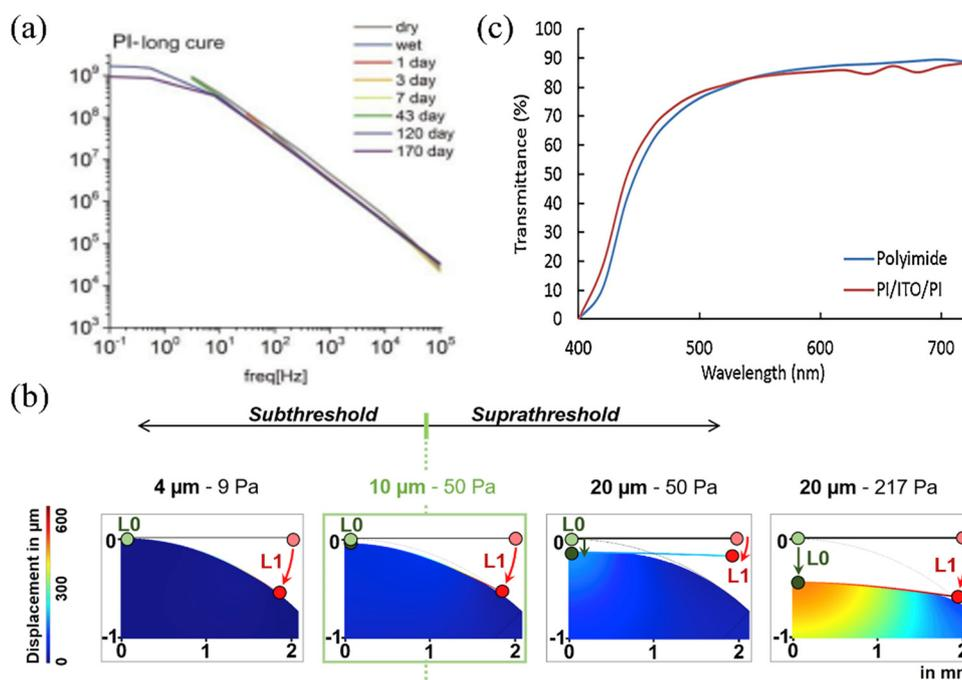
**Fig. 14** (a) Long term cured BPDA-PPD PI electrodes maintain stable impedance during long-term testing. Reprinted with permission from ref. 70. Copyright 2015, Elsevier. (b) Finite element analysis images of electrodes with varying thicknesses under diverse forces on the cerebral cortex surface. Reprinted with permission from ref. 23. Copyright 2020, Elsevier. (c) the transmittance of PI/IITO/PI ECoG electrodes. Reprinted with permission from ref. 34. Copyright 2018, Elsevier.
