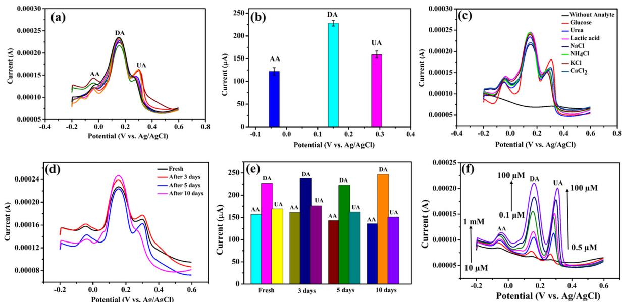
Fig. 9 Reproducibility, stability, selectivity and investigation in artificial sweat of the NiO–Ti<sub>3</sub>C<sub>2</sub>T<sub>x</sub> modified sensor: (a) reproducibility of the 8 sensors, (b) corresponding current vs. potential, (c) response of the fabricated sensor in the presence of other sweat ions and biomolecules, (d) stability of the as-fabricated biosensor, (e) corresponding current vs. number of days, and (f) response of the fabricated sensor in the presence of artificial sweat.
