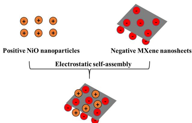
Fig. 1 Schematic illustration of the fabrication of the NiO–Ti<sub>3</sub>C<sub>2</sub>T<sub>x</sub> MXene composite.
