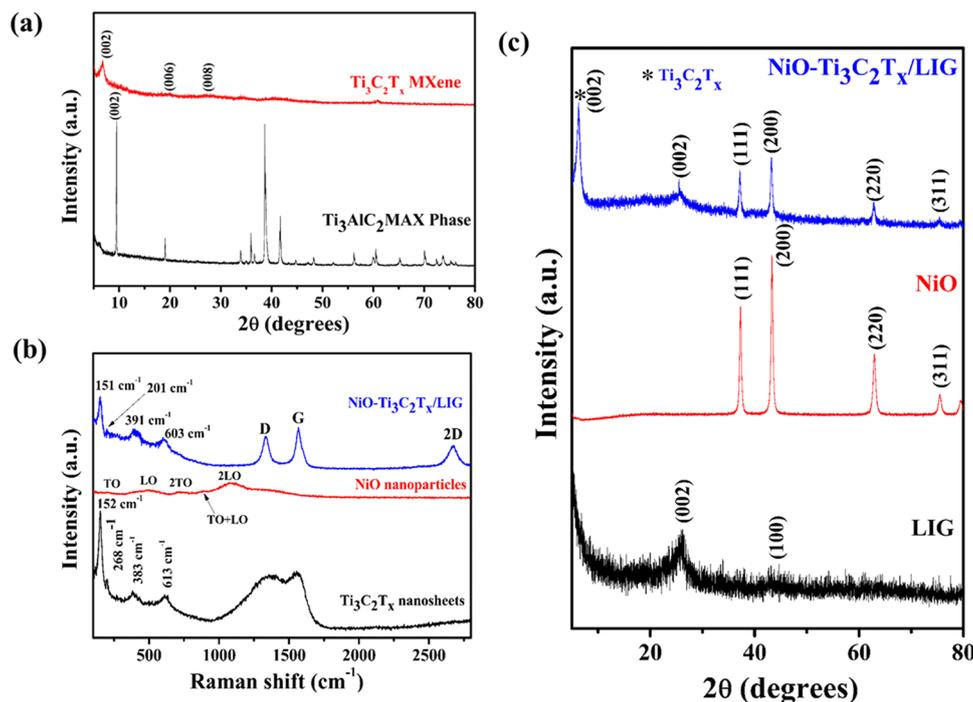
Fig. 3 (a) XRD patterns of the precursor Ti<sub>3</sub>AlC<sub>2</sub> MAX phase and delaminated Ti<sub>3</sub>C<sub>2</sub>T<sub>x</sub> MXene nanosheets. (b) Raman spectra and (c) XRD spectra of LIG, NiO nanoparticle and NiO-Ti<sub>3</sub>C<sub>2</sub>T<sub>x</sub>/LIG composite electrodes.
