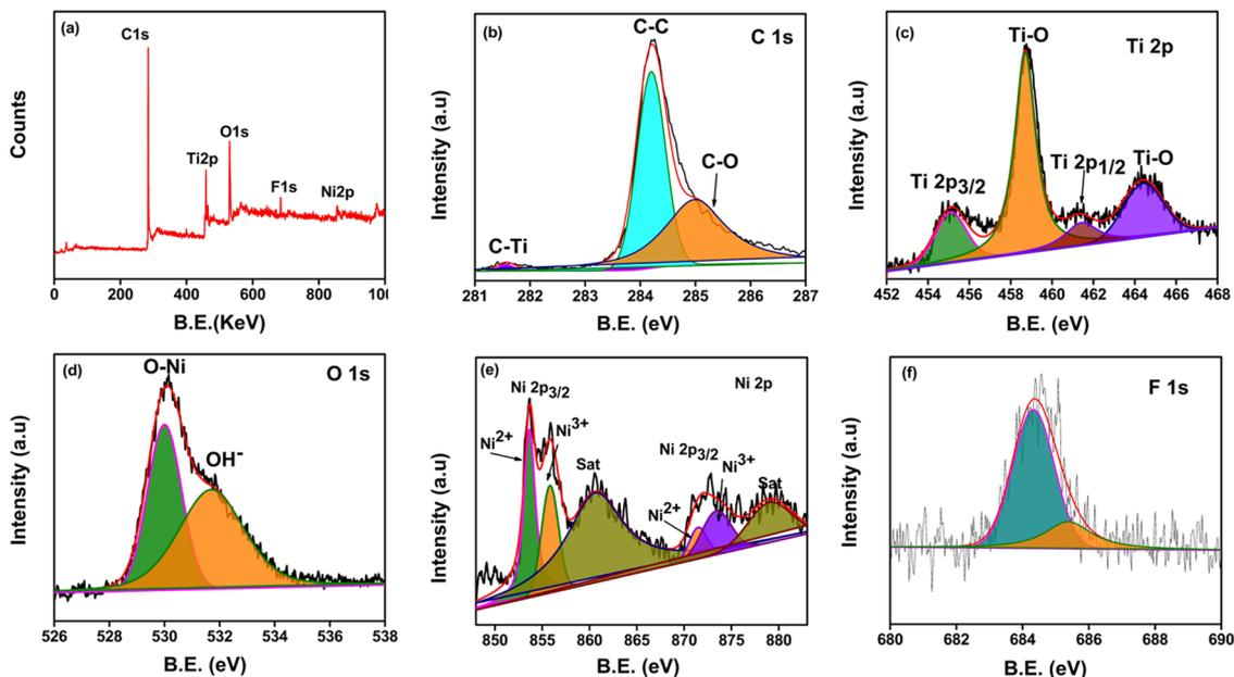
Fig. 4 (a) XPS survey spectra of the NiO–Ti<sub>3</sub>C<sub>2</sub>T<sub>x</sub>/LIG composite and high-resolution deconvoluted XPS spectra of (b) C 1s, (c) Ti 2p, (d) O 1s (e) Ni 2p, and (f) F 1s.
