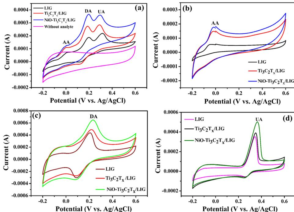
Fig. 6 Cyclic voltammograms of LIG,  $\text{Ti}_3\text{C}_2\text{T}_x/\text{LIG}$  and  $\text{NiO-Ti}_3\text{C}_2\text{T}_x/\text{LIG}$  electrodes in 0.1 M PBS (pH 7.4) containing (a) a mixture of 2 mM AA, 1 mM DA and 1 mM UA, (b) 2 mM AA, (c) 1 mM DA and (d) 1 mM UA at a scan rate of  $10 \text{ mV s}^{-1}$  compared to the response with only buffer solution.
