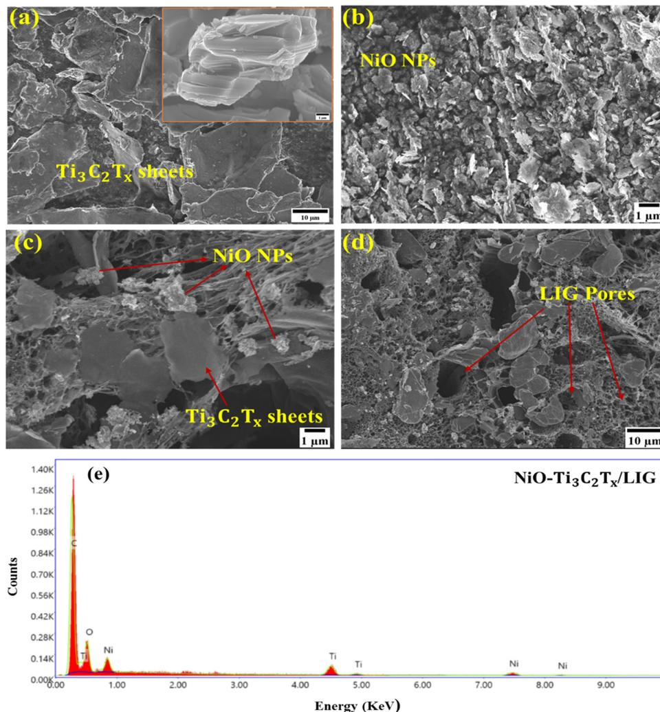
Fig. 2 FESEM images of (a)  $\text{Ti}_3\text{C}_2\text{T}_x$  MXene flakes, (b) NiO nanoparticles and (c) and (d) the  $\text{NiO-Ti}_3\text{C}_2\text{T}_x@LIG$  composite at different magnifications. (e) EDS elemental spectra of the  $\text{NiO-Ti}_3\text{C}_2\text{T}_x@LIG$  nanocomposite.
