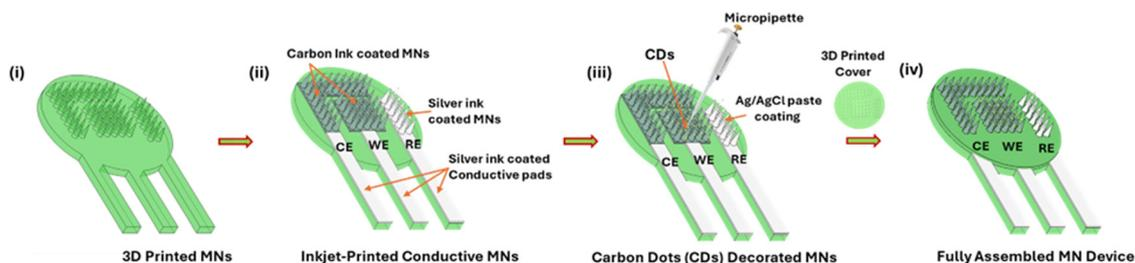
**Fig. 1** Schematic diagram of stepwise fabrication process for the three-electrode system on the tips of microneedle array using 3D printing and inkjet printing techniques: (i) 3D-printed microneedle array, (ii) inkjet-printed conductive microneedle array, (iii) carbon dots-decorated working electrode microneedles and Ag/AgCl paste coating on reference electrode microneedles, and (iv) fully assembled three-electrode system-based microneedle device.
