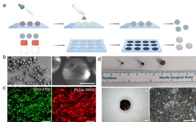
**Fig. 1** Preparation and characterization of MPs. (a) Schematic fabrication of Mg-based Janus micromotors and MPs. (b) SEM images of Mg-based Janus micromotors. Scale bars, 20  $\mu\text{m}$ . (c) Fluorescence images of the drug-loaded Mg-based Janus micromotors; GEM was labelled with FITC, and PLGA was labelled with tetramethylrhodamine isothiocyanate (TRITC). Scale bars, 100  $\mu\text{m}$ . (d) Photographs of MPs with different sizes. Scale bars, 500  $\mu\text{m}$ .
