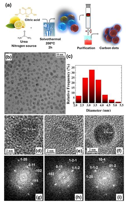
Fig. 1 (a) Schematic representation of the CD synthesis strategy, via solvothermal synthesis in water, followed by column chromatography for purification. (b) CD structural TEM analysis. Bright field overview image and (c) corresponding size distribution. (d)—(f) High resolution images of three representative single particles. (g)-(i) Fast Fourier transform (FFT) spectrum of the dots selected above in panels (d)-(f), respectively.
