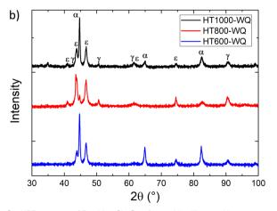
Fig. 2 XRD spectra of Fe-Mn-Si-Cu after cold rolling and heat treatment at various temperatures followed by (a) furnace cooling; (b) water quenching
