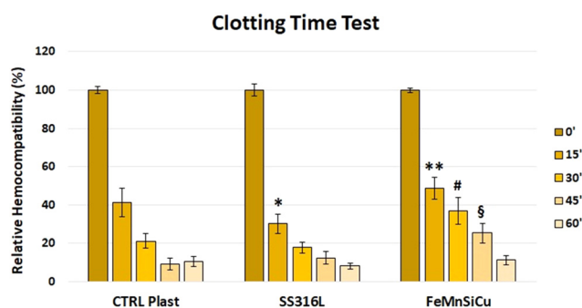
Fig. 14 Clotting time test performed on SAE 316L grade stainless steel (SS316L), Fe–Mn–Si–Cu (FeMnSiCu) compared to the control condition (CTRL Plast). * p < 0.01 vs. CTRL Plast 15' and p < 0.001 vs. FeMnSiCu 15'; ** p < 0.01 vs. CTRL Plast 15'; # p < 0.001 vs. CTRL Plast and SS316L 30'; § p < 0.001 vs. CTRL Plast and SS316L 45'.
