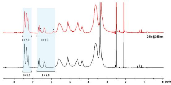
Fig. 7  $^{1}$ H-NMR spectra of the CS2 starch ether in DMSO- $d_6$  before and after 24 h UV exposure at  $\lambda \sim 365$  nm. Shaded areas highlight changes in the spectra and \* indicates new peaks; relevant integrals are indicated (I).
