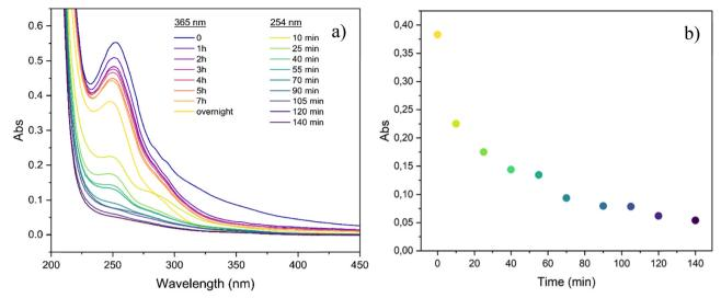
Fig. 6 (a) UV-Vis spectra of CS1 sample after exposure at  $\lambda \sim 365$  nm and, subsequently, at  $\lambda = 254$  nm and (b) maximum absorption plotted against UV irradiation time at  $\lambda = 254$  nm.
