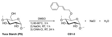
Scheme 3 Starch etherification with cinnamyl moieties (CINN-Cl, cinnamyl chloride). Three different molar equivalents of NaOH and cinnamyl chloride were used, affording products CS1-CS3 with different degrees of substitution.
