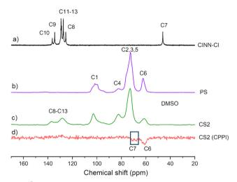
Fig. 4 <sup>13</sup>C CPMAS NMR of (a) CINN-Cl, (b) pristine yuca starch (PS), (c) cinnamyl starch CS2, and (d) <sup>13</sup>C CPPI NMR spectra of CS2 sample (cinnamyl methylene carbons involved in the ether linkage are highlighted).
