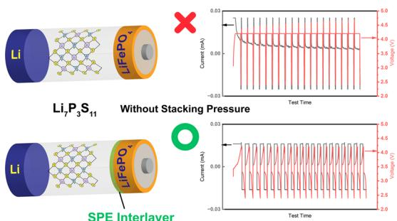
**Synergy of metal halide doping and a polymeric interface enables improved electrochemical performance of all solid-state Li batteries**
