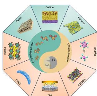
**Taming polysulfide shuttle and lithium dendrites in lithium–sulfur batteries via all-/quasi-solid-state electrolytes: recent progress and future prospects**
