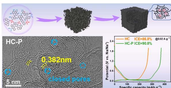
**Stepwise crosslinking–activation to create a closed pore structure of hard carbon for boosted sodium energy**
