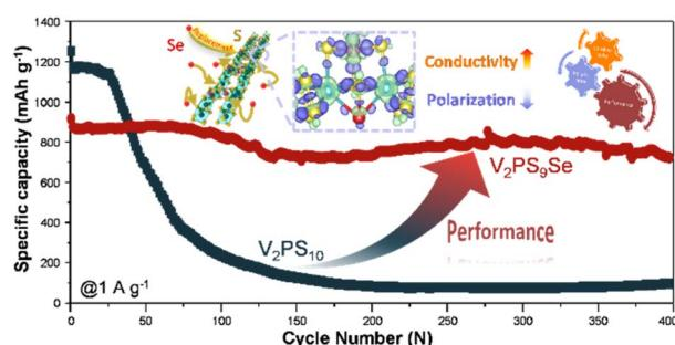
**A novel 1D van der Waals V<sub>2</sub>PS<sub>x</sub>Se<sub>10-x</sub> ( $x = 7\text{--}10$ ) anode for enhanced electrochemical kinetics and high-rate performance via Se alloying in lithium-ion batteries**
