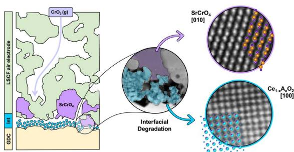
**Atomic-scale insights into air electrode degradation after 10 years of fuel cell stack operation**
