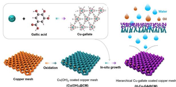
**A hierarchical Cu-gallate-based mesh membrane for oil/water separation**
