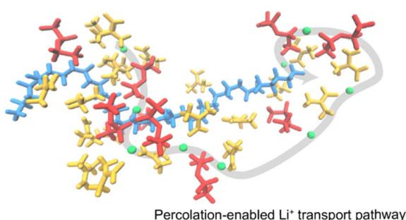
**Percolation-enabled long-range ion transport to achieve conductivity leap in PVDF-based electrolytes**
