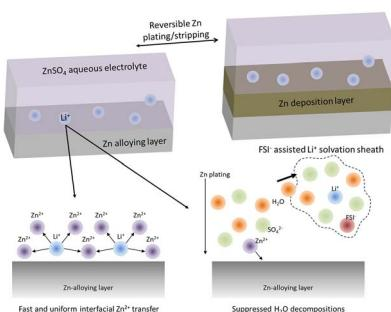
**Lithium ion mediated interfacial transfer and solvation structure enable stable zinc-alloying interface for aqueous zinc battery**
