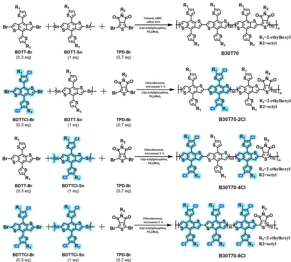
**Scheme S1** Synthetic scheme of B30T70-XCl (X = 0, 2, 4, 6).
