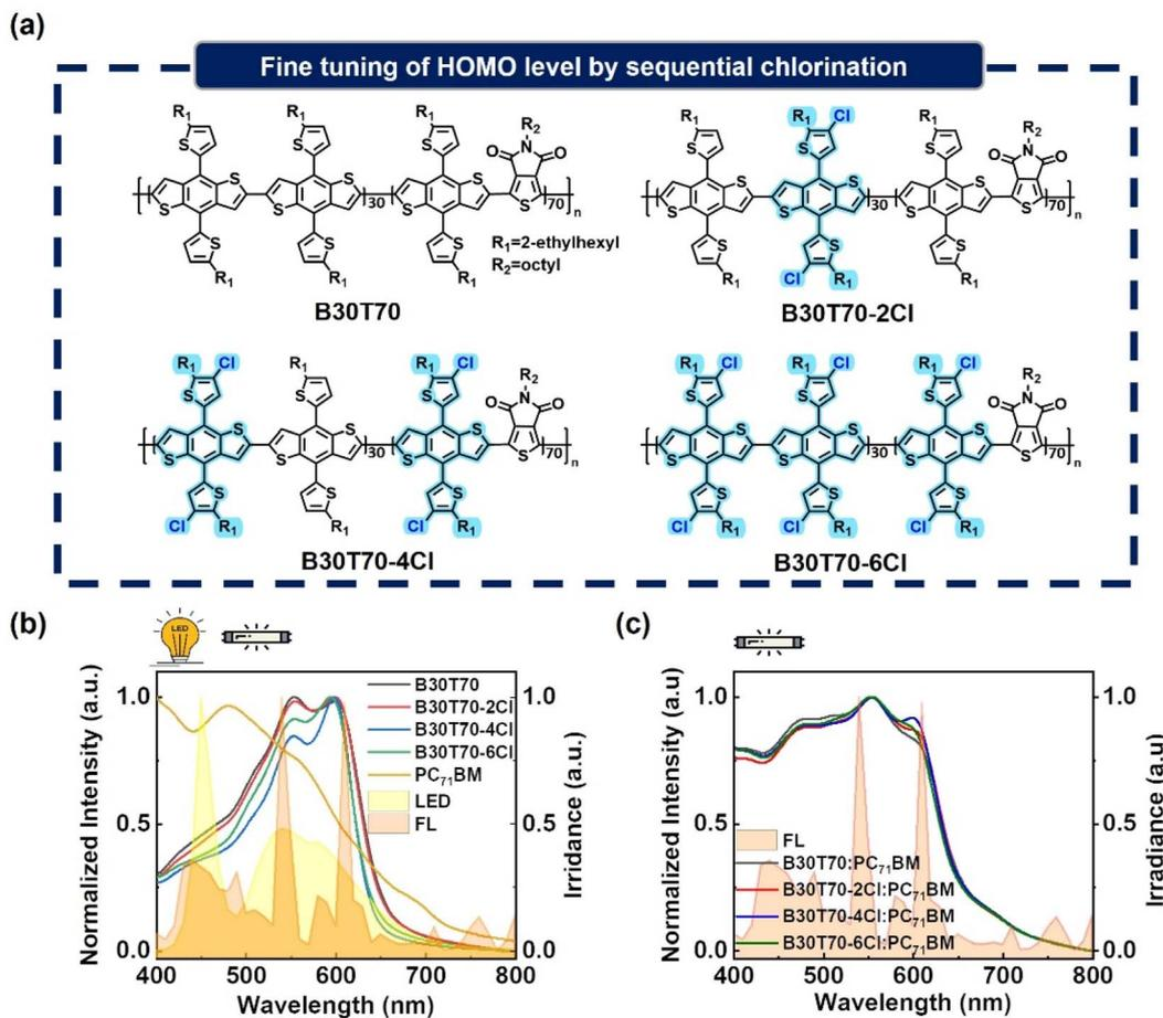
**Fig. 1** (a) Chemical structures of B30T70-XCl (X = 0, 2, 4 and 6), (b) absorption spectra of pristine polymer donors, acceptor PC<sub>71</sub>BM, and illumination spectra of indoor light sources (LED and FL), and (c) absorption spectra of blend films.
