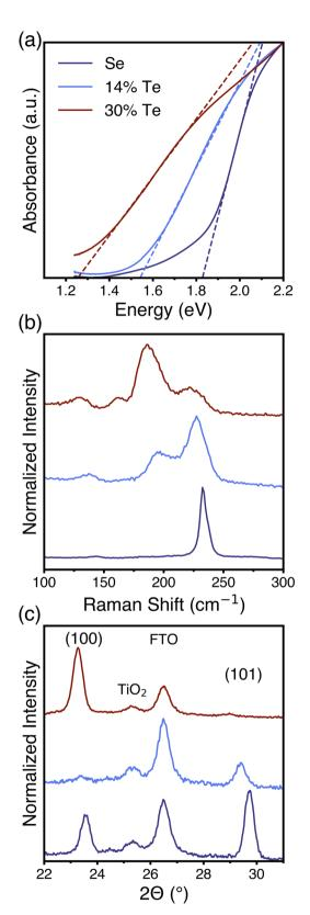
Fig. 4 Film characterization. (a) UV-Vis absorbance (b) Raman and (c) XRD for varying Te concentration. For this figure and those that follow, the dark blue curve corresponds to pure Se, the light blue corresponds to 14% Te, and the red curve corresponds to 30% Te.
