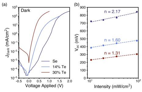
Fig. 6 Dark J-V electrical characterization and illumination-dependent  $V_{\infty}$  as a function of Te concentration. (a) Semi-log J-V characteristics of cells measured under dark conditions. (b) Illumination-dependent  $V_{oc}$  and ideality factor fit.
