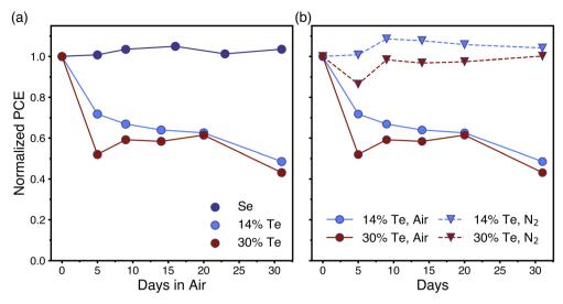
Fig. 7 Stability of Unencapsulated Devices. (a) Normalized PCE over time for devices stored in dark in air and remeasured over time. (b) Comparing the stability of  $Se_{1-x}Te_x$  cells stored in air vs. stored in an  $N_2$ -filled glovebox over time. All devices are measured in air.
