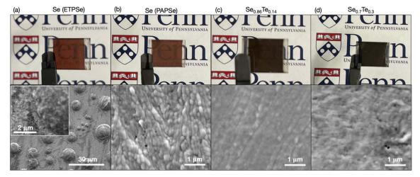
Fig. 2 Optical and Electron Microscope Images of Films. Camera (top row) and SEM (bottom row) images of (a) Se processed from ETPSe, (b) Se processed from PAPSe, (c) 14% Te, and (d) 30% Te films. The camera images are taken from the bottom side of the 20 mm  $\times$  15 mm TiO<sub>2</sub>/FTO/ glass substrate.
