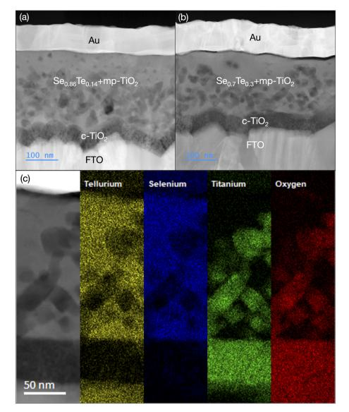
Fig. 3 Cross sectional scanning TEM (STEM) analysis. (a) High-Angle Annular Dark Field STEM (HAADF-STEM) images of (a) 14% Te and (b) 30% Te films, indicating absorber layer thicknesses of approximately 200 nm. The ultrathin  $MoO_x$  layer is present in all images but is not labeled in the images for readability. (c) X-STEM image and EDS maps of Te, Se, Ti, and O for the 30% Te film confirming uniform alloying and full infiltration of the mesoporous (mp)-TiO<sub>2</sub> layer.
