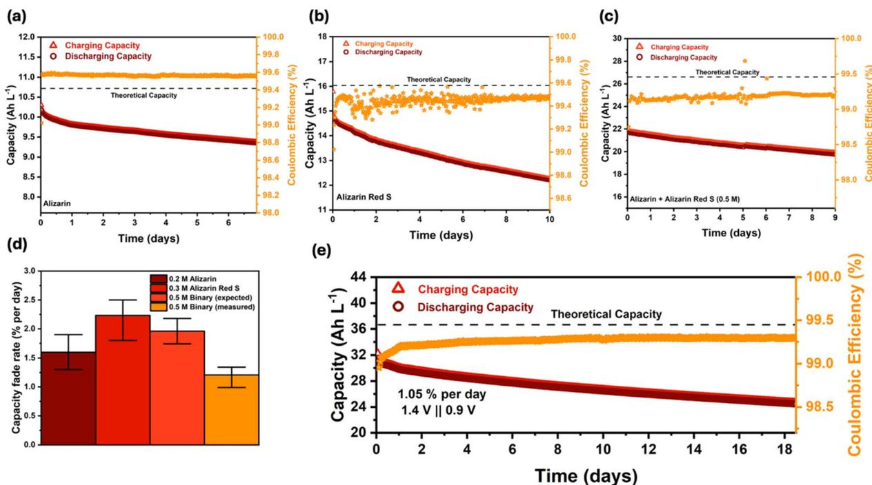
Fig. 2 Long-term RFB cycling tests of (a) 0.2 M alizarin in 1.4 M KOH, (b) 0.3 M alizarin red S in 1.6 M KOH, and (c) 0.5 M binary negolyte (0.2 M alizarin + 0.3 M alizarin red S) in 2 M KOH. (d) Capacity fade rate comparison of all cells with 3 repetitions for each battery. (e) Cycling of 0.7 M binary electrolyte (0.3 M alizarin + 0.4 M alizarin red S) in 2.4 M KOH. All cells were operated at pH 14, with Nafion 117 membranes and ferro-/ferricyanide as the posolyte.
