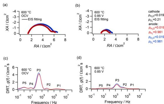
**Fig. 5** Nyquist plots of the impedance and DRT spectra of SOFCs at 600 °C when the gas at the anode is replaced from light to heavy hydrogen. Impedance spectra under (a) OCV and (b) polarization states (0.85 V). DRT spectra under (c) OCV and (d) polarization states (0.85 V).
