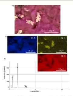
Fig. 4 EDX results: (A) ChemiSEM image of Ag/Al 550, (B) elemental maps of oxygen, aluminum and silver, and (C) EDX spectrum.
