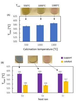
Fig. 10 Temperature of the maximum soot combustion rate determined for: (A) chromium-doped supports calcined at different temperatures and (B) supports calcined at 1300 °C and the respective catalysts.
