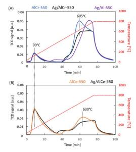
Fig. 8  $CO_2$ -TPD study results of: (A) AlCr-550, Ag/AlCr-550 and Ag/Al-550 and (B) AlCe-550 and Ag/AlCe-550.
