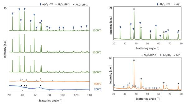
Fig. 3 Diffraction patterns of (A) the alumina supports calcined at different temperatures, (B) Ag/Al 1000 and (C) Ag/Al 900.
