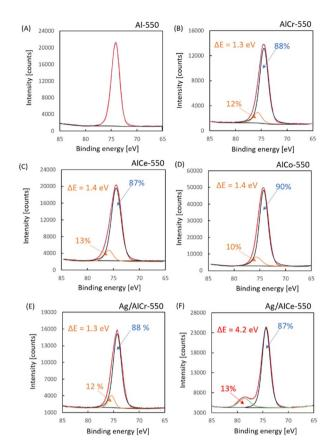
Fig. 7 The detailed Al 2p regions of: (A) Al-550, (B) AlCr-550, (C) AlCe-550, (D) AlCo-550, (E) Ag/AlCr-550 and (F) Ag/AlCe-550; measurement points – red solid curve, envelope – blue dotted curve.
