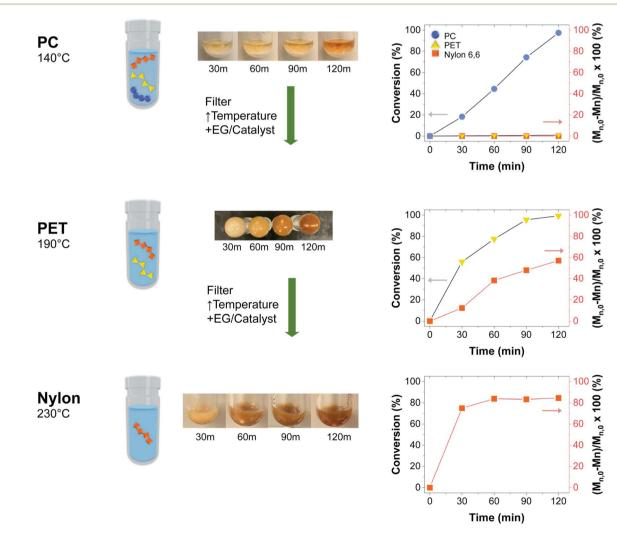
Fig. 3 Changing temperature enables the selective and seguential deconstruction of PC. PET, and Nylon 6.6.
