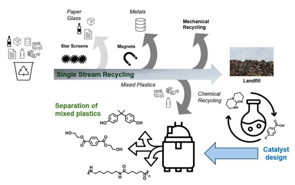
Fig. 1 Chemical recycling can be used to process mixed plastics after metals, papers, and glass have been sorted out from single stream recycling feedstocks. Selective glycolysis can process mixed plastic streams. Landfill photograph by Emmet from Pexels.com. Energy and catalyst icons: Flaticon.com.
