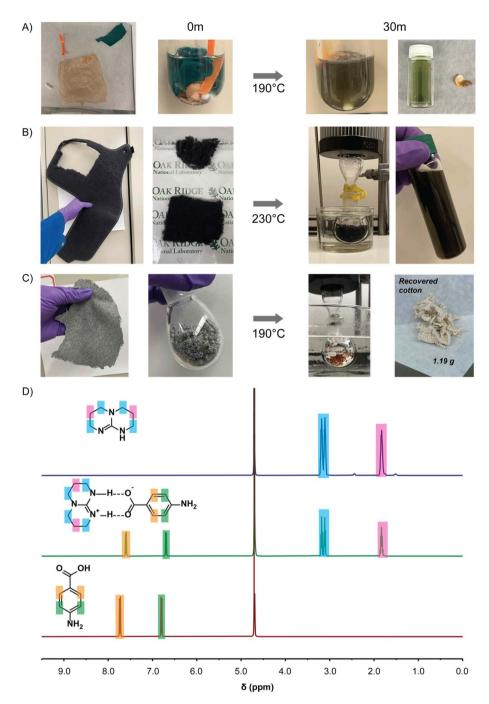
Fig. 4 (A) Deconstruction of mixed plastics and PET fabric achieved in 30 min and leaves unreactive plastics behind. (B) Deconstruction of fibers from automobile floor mat. (C) Deconstruction of 50:50 polyester: cotton blend clothing. (D) Stacked <sup>1</sup>H NMR spectra of TBD, PABA, & TBD: PABA.
