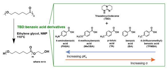
Scheme 1 Chemical deconstruction of PCL using TBD: benzoic acid derivatives.
