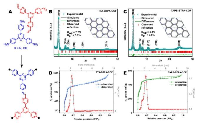
Fig. 1 (A) Synthetic scheme of TTA-BTPA-COF and TAPB-BTPA-COF. The PXRD patterns with corresponding simulated diffractogram and Pawley refinements of (B) TTA-BTPA-COF and (C) TAPB-BTPA-COF. N<sub>2</sub> sorption isotherms and pore size distribution of (D) TTA-BTPA-COF and (E) TAPB-BTPA-COF.
