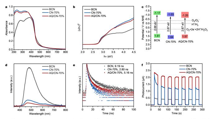
Fig. 3 (a) UV-Vis DRS and (b) Tauc plot of BCN, CN-70% and AQ/CN-70%, (c) band structure alignments of BCN, CN-70% and AQ/CN-70%, (d) steady-state PL spectra, (e) time-resolved transient PL spectra and (f) transient photocurrent responses of BCN, CN-70%, and AQ/CN-70%.
