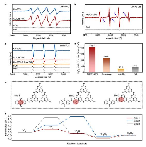
Fig. 5 (a)  $\cdot O_2^-$ , (b)  $\cdot OH$  and (c)  $^1O_2$  radical adduct signals in EPR spectra of BCN, CN-70%, AQ/CN-70% and CN-70% with the addition of BQ, (d) H<sub>2</sub>O<sub>2</sub> production rates of AQ/CN-70% with different radical scavengers, (e) schematic illustration of potential <sup>1</sup>O<sub>2</sub> reaction sites, and (f) free energy diagrams for H<sub>2</sub>O<sub>2</sub> formation pathways at distinct reaction sites on AQ/CN-70%.
