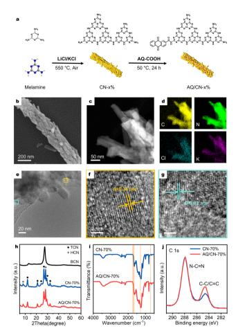
Fig. 1 (a) Schematic illustration of the synthesis route for AQ/CN-x%, (b) SEM image of AQ/CN-70%, (c and d) HAADF-STEM and related EDX elemental mapping images of AQ/CN-70%, (e-g) TEM and HRTEM of AQ/CN-70%, with lattice fringes from regions marked by coloured boxes in (e), (h) XRD patterns of BCN, CN-70%, and AQ/CN-70%, (i) FTIR spectra of CN-70% and AQ/CN-70%, and (j) XPS spectra of C 1s for CN-70% and AQ/CN-70%.
