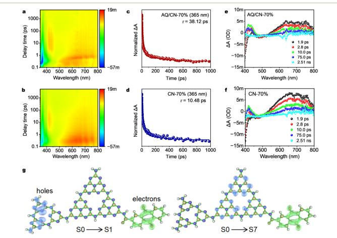
Fig. 4 2D mapping TA spectra of (a) AQ/CN-70% and (b) CN-70%, TA spectra signals on the fs-ns timescales of (c) AQ/CN-70% and (d) CN-70%, decay kinetic curves of (e) AQ/CN-70% and (f) CN-70%, and (g) the excited state information of AQ/CN-70% from DFT calculations.
