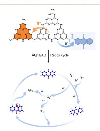
Fig. 6 Charge transfer and AQ/ $H_2AQ$  redox cycle mechanism for photocatalytic  $H_2O_2$  synthesis on the AQ/CN-x% catalyst.
