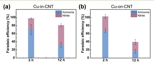
Fig. 4 Stability study of (a) Cu-in-CNT (2 wt%) (at -1.2 V) and (b) Cu-on-CNT (12 wt%) (-1.3 V) towards nitrate reduction at 2 h and 12 h in phosphate buffer (pH 7.3) containing 0.1 M KNO<sub>3</sub>. Error bars represent standard deviations from n=3 samples.
