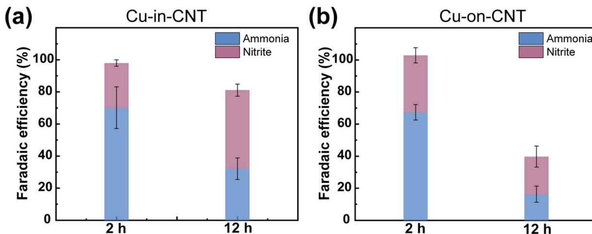
Fig. 4 Stability study of (a) Cu-in-CNT (2 wt%) (at  $-1.2$  V) and (b) Cu-on-CNT (12 wt%) ( $-1.3$  V) towards nitrate reduction at 2 h and 12 h in phosphate buffer (pH 7.3) containing 0.1 M  $\text{KNO}_3$ . Error bars represent standard deviations from  $n = 3$  samples.
