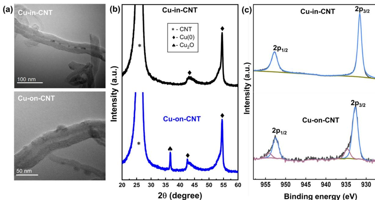
Fig. 5 Post-electrolysis characterization of catalysts. (a) TEM images of Cu-in-CNT and Cu-on-CNT. (b) XRD of Cu-in-CNT and Cu-on-CNT. (c) XPS of Cu-in-CNT and Cu-on-CNT. Deconvolution peaks correspond to Cu(II) (red line), Cu(I)/Cu(0) (blue line) and baseline (green).
