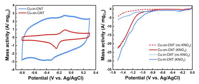
Fig. 2 (a) Cyclic voltammograms of Cu-on-CNT (2 wt%) and Cu-in-CNT (12 wt%) recorded in 0.1 M phosphate buffer (pH 7.3) at a scan rate of 30 mV s<sup>-1</sup>. (b) Voltammogram of Cu-on-CNT and Cu-in-CNT in the presence and absence of 0.1 M KNO<sub>3</sub>, recorded in 0.1 M phosphate buffer (pH 7.3). Scan rate: 10 mV s<sup>-1</sup>. The current is normalized to the mass of Cu obtained from redox peaks of Cu.
