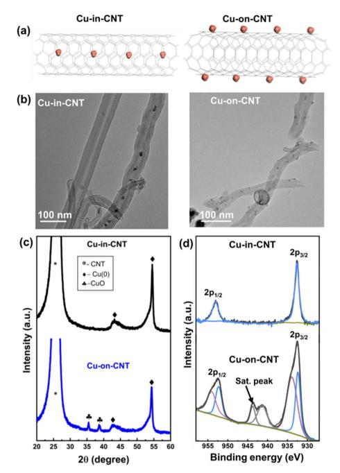
Fig. 1 (a) Schematic illustration of Cu-in-CNT and Cu-on-CNT. (b) TEM images of Cu-in-CNT and Cu-on-CNT. (c) XRD of Cu-in-CNT and Cu-on-CNT. on-CNT. (d) X-ray photoelectron spectra of Cu-in-CNT and Cu-on-CNT. Deconvoluted peaks correspond to Cu(i)/Cu(0) (blue), Cu(ii) (red) and baseline (green).
