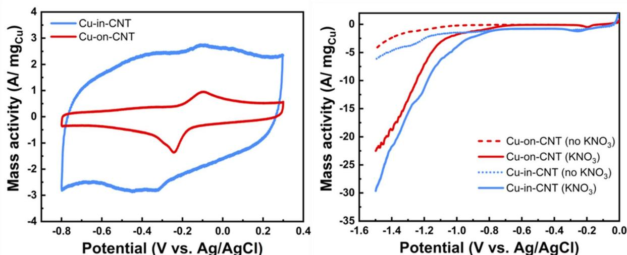
Fig. 2 (a) Cyclic voltammograms of Cu-on-CNT (2 wt%) and Cu-in-CNT (12 wt%) recorded in 0.1 M phosphate buffer (pH 7.3) at a scan rate of  $30 \text{ mV s}^{-1}$ . (b) Voltammogram of Cu-on-CNT and Cu-in-CNT in the presence and absence of 0.1 M  $\text{KNO}_3$ , recorded in 0.1 M phosphate buffer (pH 7.3). Scan rate:  $10 \text{ mV s}^{-1}$ . The current is normalized to the mass of Cu obtained from redox peaks of Cu.
