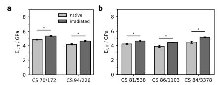
Fig. 3 Nanoindentation of 0-30% TEGABS|CS films before and after UV irradiation. Illustration of the influence of UV-light on E<sub>r,IT</sub> (a and b) in 20% TEGABS|CS films with varying DDA (a) and DP (b) before and after UV irradiation ( $\lambda_{\rm exc} = 365$  nm, dose of 33 J cm<sup>-2</sup>). Notably, the Student's ttests were conducted at a significance level of 0.01 (\* = p < 0.01).
