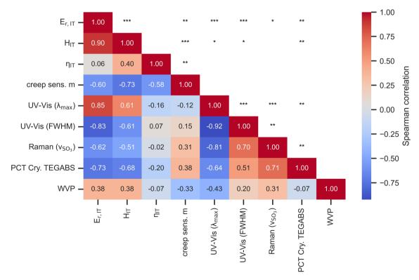
Fig. 8 Spearman correlation matrix of the (mean) values of the spectroscopic and mechanical variables measured in their native states. It should be noted that the significance levels, indicated by p-values, are shown in the upper triangle with \* = p < 0.05, \*\* = p < 0.01 and \*\*\* = p < 0.001.
