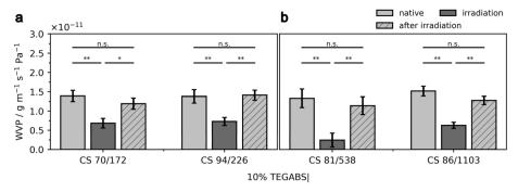
Fig. 4 Water vapor permeability measurements of 10% TEGABS|CS membranes in cup tests. Influence of UV light (365 nm, 55 mW cm<sup>-2</sup>) on the WVP of DP < 300 (a) and DP > 500 (b) membranes with 10% TEGABS|CS. Notably, the Student's t-tests were conducted using a significance level of \* = p < 0.1 (probability of a type-II error ( $\beta$ ) < 0.35), \*\* = p < 0.05 and \*\*\* = p < 0.01.
