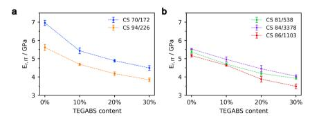
Fig. 2 Nanoindentation of native 0–30% TEGABS|CS films. Influence of different TEGABS concentrations as well as the DDA (a) and DP (b) of chitosan on  $E_{\rm r,IT}$ .
