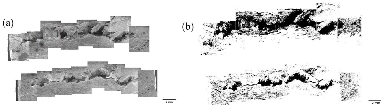
Fig. 5 (a) SEM micrograph showing the crack area before and after healing; (b) ImageJ analysis of the corresponding area. For Al40Sn1.5NiTi, the crack area before healing was measured as 27.3 mm<sup>2</sup>, which reduced to 5.2 mm<sup>2</sup> after healing, resulting in a 81% reduction in the crack area (size of the scale bar: 2 mm).
