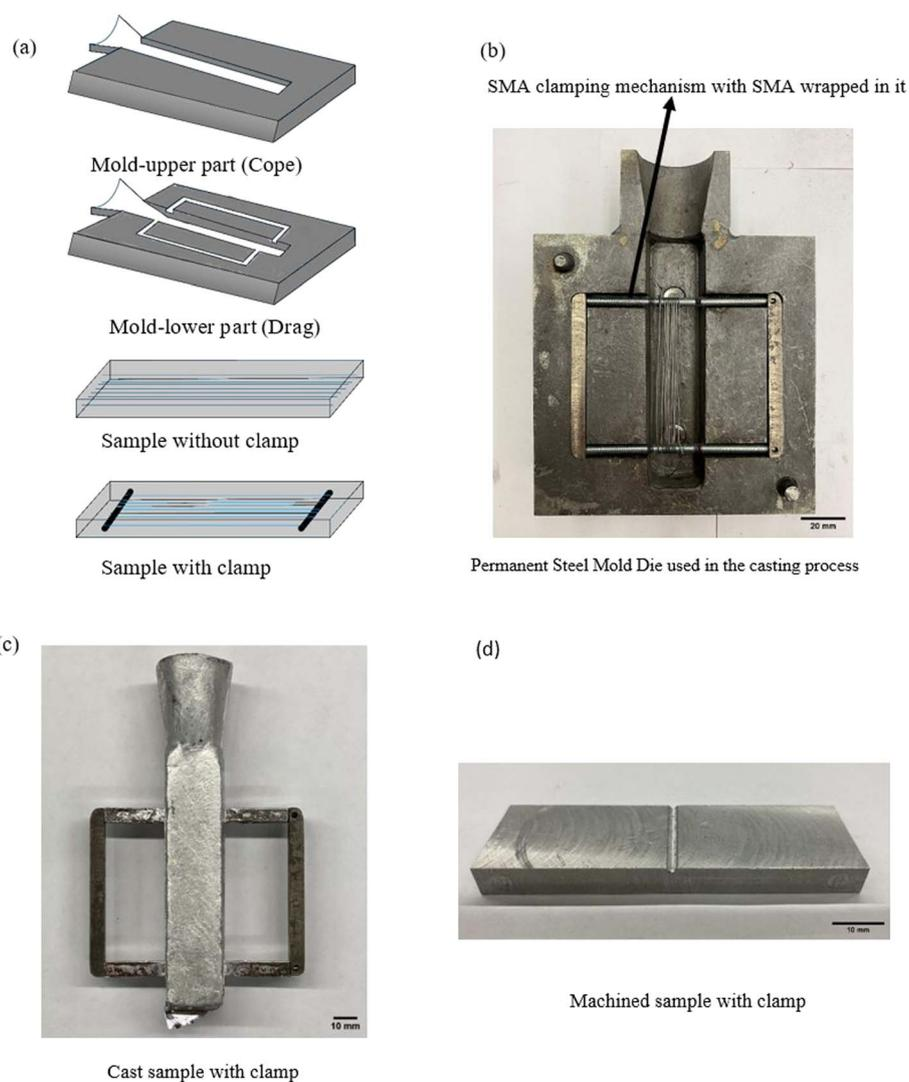
**Fig. 1** (a) Mold and sample design for casting self-healing aluminum composites with *in situ* low-melting-point phase; (b) permanent steel mold die used in the casting process; (c) cast sample with clamping mechanism; (d) machined sample with clamping mechanism.
