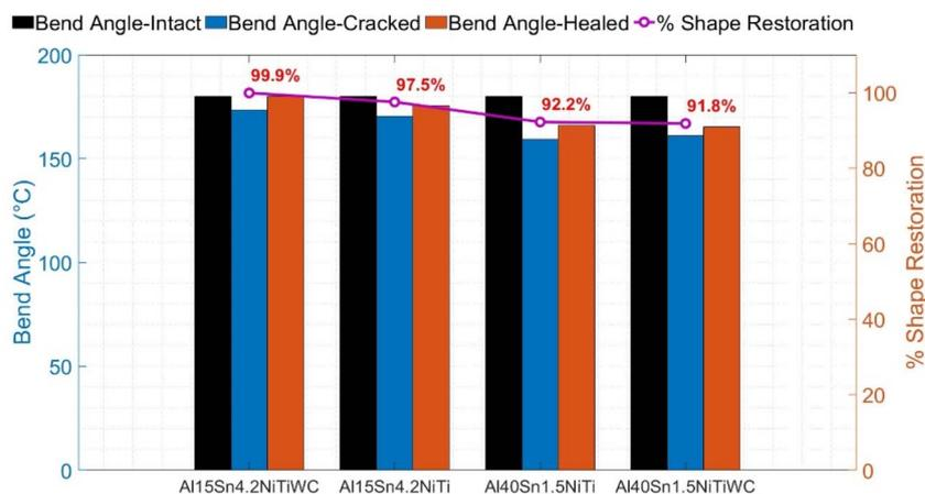
Fig. 6 Shape restoration of self-healing aluminum–tin (Al–Sn) composites: (a) optical images of samples before and after self-healing; (b) graph comparing shape restoration.
