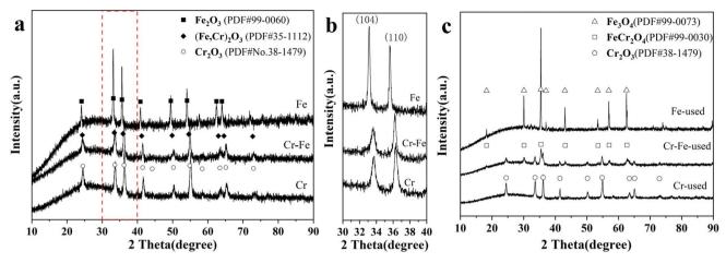
Fig. 3 (a) XRD patterns of fresh FeCrO<sub>x</sub> catalysts, (b) the magnified portion of the curve in the 30–40° range in (a), and (c) XRD patterns of used FeCrO<sub>x</sub> catalysts.
