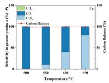
Fig. 2 Selectivity in gaseous products and carbon balance of (a) Cr-Fe, (b) Cr, and (c) Fe.
