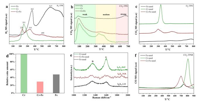
Fig. 9 (a)  $H_2$ -TPR of fresh FeCrO<sub>x</sub> samples, (b)  $CO_2$ -TPD of FeCrO<sub>x</sub> samples, (c)  $O_2$ -TPO and (f)  $CO_2$ -TPSR of the used FeCrO<sub>x</sub> samples, (d) the estimated relative coke deposition on the catalyst from (c), and (e) Raman spectra of used  $FeCrO_x$  samples in the wavenumber range of 1000- $2000 \text{ cm}^{-1}$
