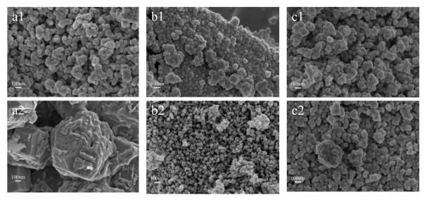
Fig. 4 SEM images of FeCrO<sub>x</sub> catalyst samples (1) before and (2) after the reaction: (a) Fe, (b) Cr-Fe, and (c) Cr.
