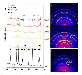
Fig. 8 In situ SR-XRD (a) patterns of the Cr-Fe catalyst during the CO<sub>2</sub>-ODHE reaction and 2D images of (b) fresh catalyst (c) after pretreatment at 450 °C in 50% H<sub>2</sub>/Ar and (d) at 650 °C in the reaction gases  $(CO_2/C_2H_6/Ar = 10/10/20 \text{ mL min}^{-1})$ .
