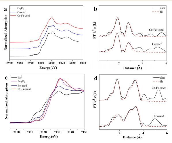
Fig. 7 Cr K-edge: (a) XANES profiles and (b) EXAFS fitting results; Fe K-edge: (c) XANES profiles and (d) EXAFS fitting results in R space of used FeCrO<sub>x</sub> catalysts.
