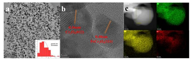
Fig. 5 (a) TEM, (b) high-resolution TEM images and (c) elemental mapping images of the Cr-Fe-used catalyst.
