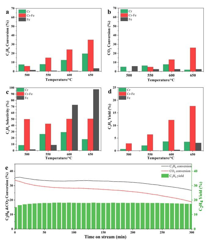
Fig. 1 Catalytic performance of the CO<sub>2</sub>-ODHE reaction of Cr, Cr-Fe, and Fe. (a)  $C_2H_6$  conversion, (b)  $CO_2$  conversion, (c)  $C_2H_4$  selectivity, (d)  $C_2H_4$  yield, and (e) stability at 650 °C of Cr-Fe samples (space velocity: 24 000 mL  $g_{cat}^{-1} h^{-1}$ ).
