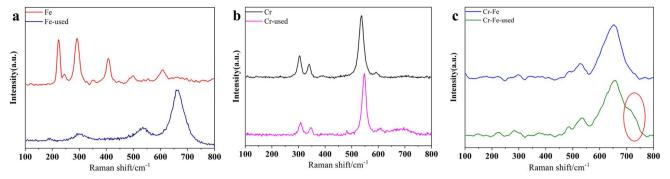
Raman patterns of (a) Fe, (b) Cr, and (c) Cr-Fe catalysts before and after the reaction.
