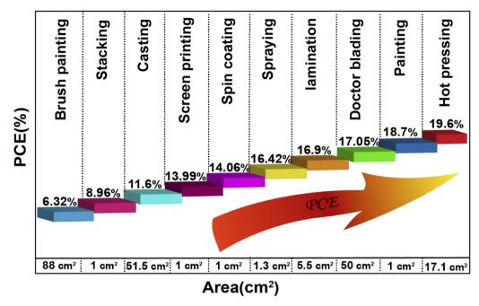
Fig. 4 Top PCEs measured for large-area (≥1 cm<sup>2</sup>) C-PSCs using various scalable deposition methods for carbon electrodes.<sup>42,80,98–105</sup>
