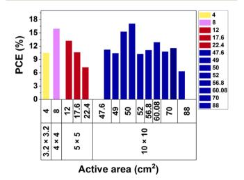
Fig. 8 Scaling-up process of C-PSCs. PCEs of large-area C-PSCs and C-PSMs as a function of active area.
