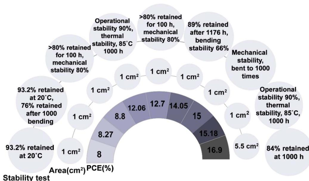
Fig. 7 Stability achievements for large area ( $\geq 1 \text{ cm}^2$ ) rigid C-PSCs and FC-PSCs.
