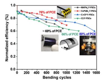
Fig. 6 Bending test of FC-PSCs.
