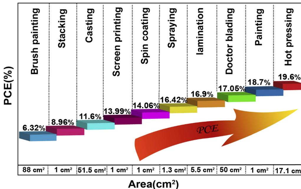
Fig. 4 Top PCEs measured for large-area ( $\geq 1$  cm<sup>2</sup>) C-PSCs using various scalable deposition methods for carbon electrodes.<sup>42,80,98–105</sup>
