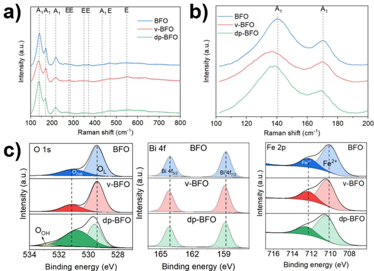
Fig. 3 (a) Raman spectra and (b) magnified Raman spectra in the region 100 – 200 cm<sup>-1</sup> for the pristine BFO, v-BFO, and dp-BFO thin films. (c) O 1s, Bi 4f and Fe 2p XPS spectra of pristine BFO, v-BFO, and dp-BFO.
